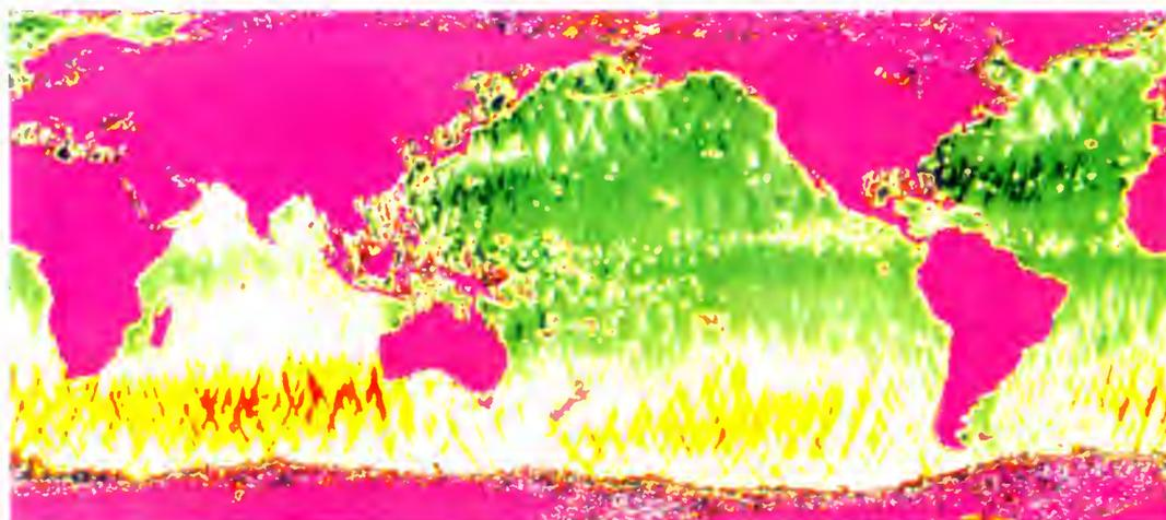
Figure 8. Significant wave height from radar altimetry
