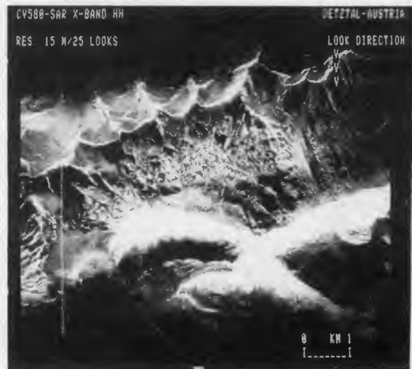
Figure 8. Display of the digitally processed SAR-580 data of the Oetzal site, 5x5 pixels averaged.
