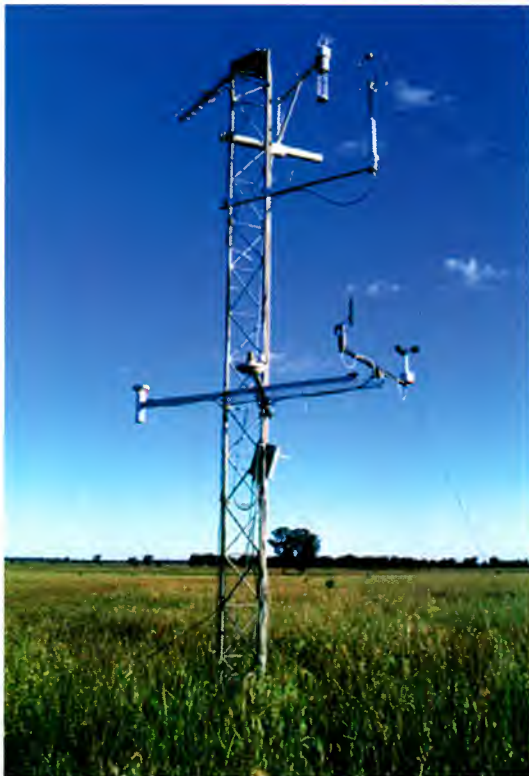
Flux towers monitor exchanges of CO 2 , water vapour and energy between land and atmosphere.
