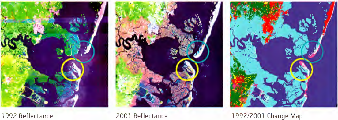
Erosion and accretion along barrier islands near Beach Heaven, New Jersey, USA. This area on the New Jersey shoreline contains small but notable changes in the barrier island complex due to wave action. Although only 1.67% of all pixels in this area were identified as changed, there are economic consequences when high value urban real estate from Beach Haven, NJ, is transported down the coast.
