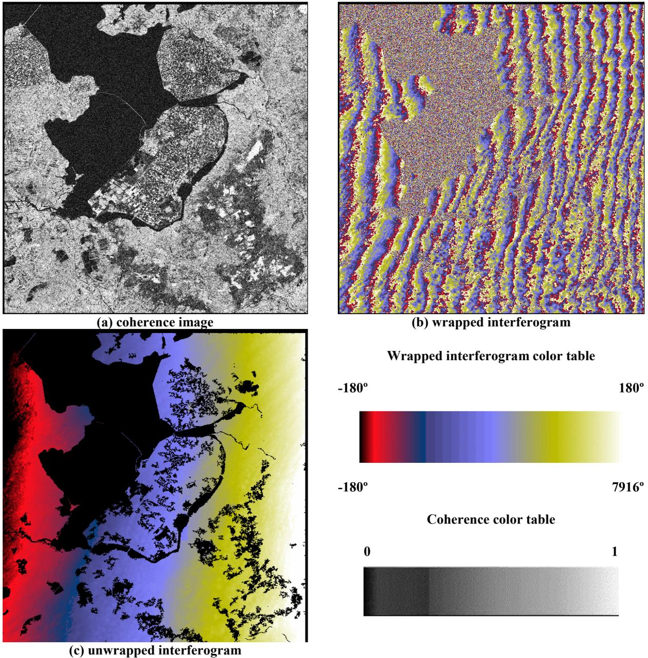
Figure 2: coherence and interferogram images from the reference pair E2\_VMP/E1\_VMP
