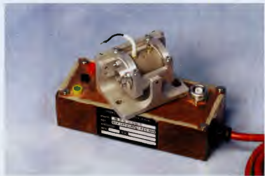
Q-Switch Driver (MMS)
