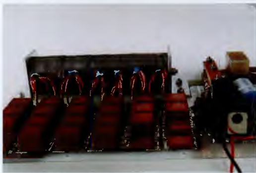
Diode Power Supply (DSS)
