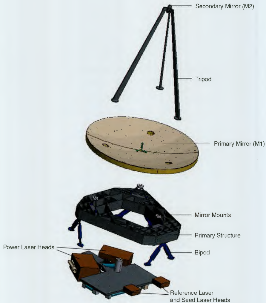
Figure 6.25. Opto-mechanical architecture of instrument core (star tracker not shown)
