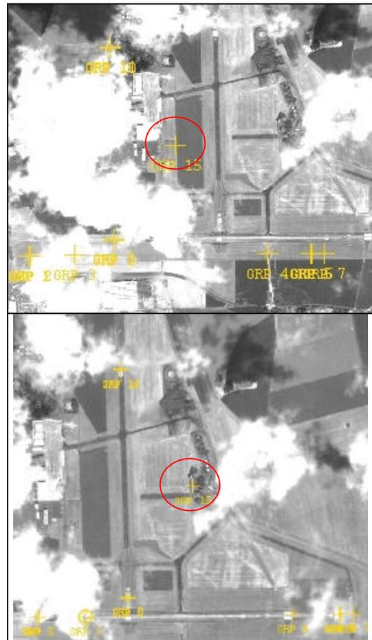
Figure 14. The upper image is from product processed prior to correction of across track and along track errors. The bottom image is from product processed after processor update. Ground control point pattern overlaid the both image. GCP 15 surrounded with red circle matches the exact geo location on the bottom image, this is not the case for the upper image.
