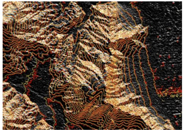
Figure 17. DEM Piemonte (Italy) in background, altitude curves, PRISM (red), SPOT (yellow).
