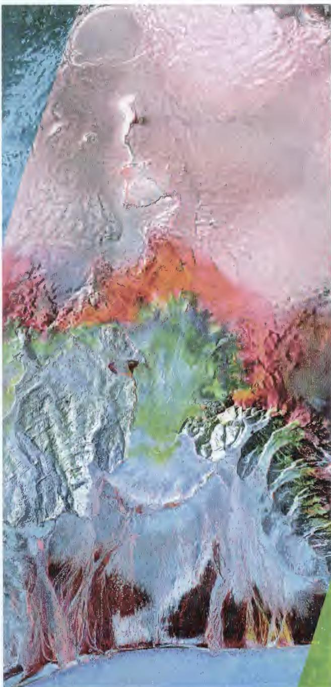
Figure 17: Geocoded terrain corrected multitemporal ERS-1/2 mosaic (desc.), acquired on Oct. 21, Oct. 22 and Nov. 7, 1996 (BGR).
