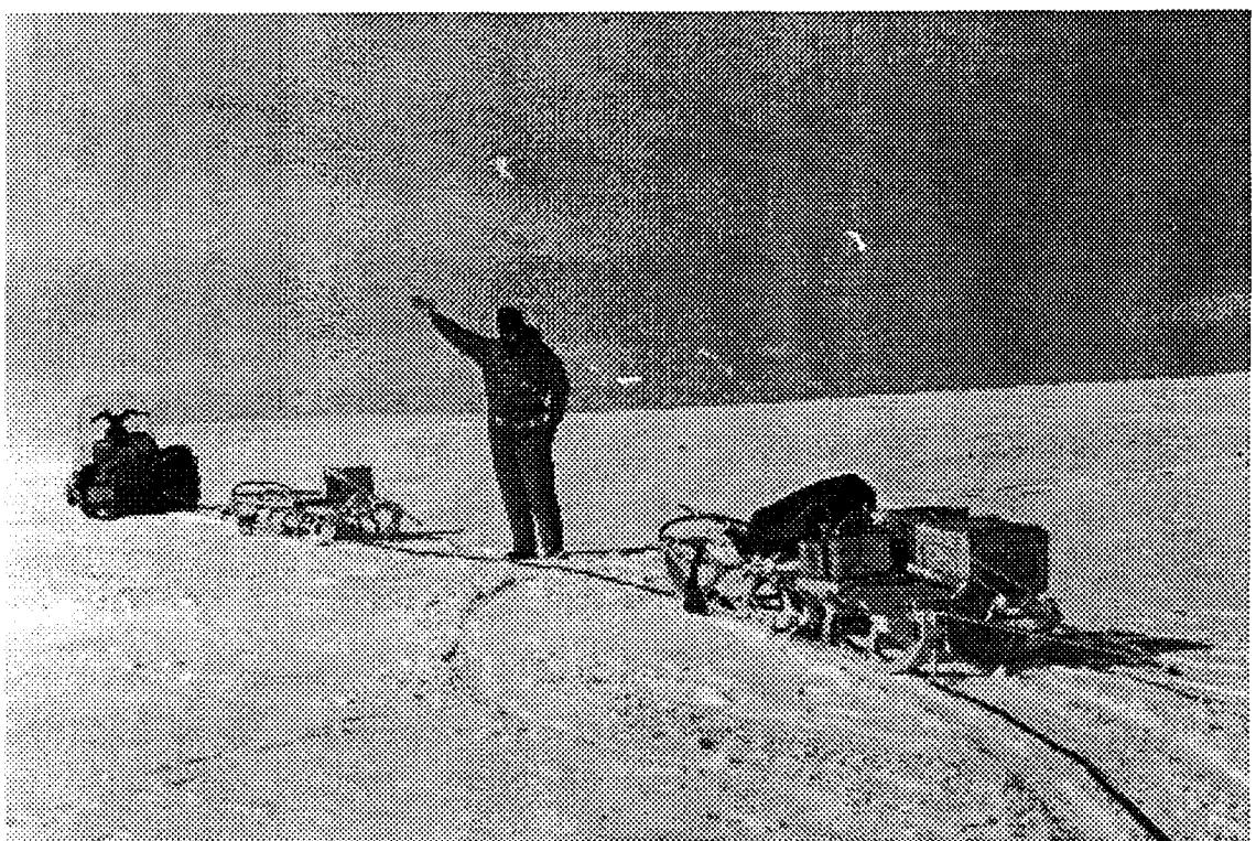
Fig. 3. Ground-based radio echo-sounding measurements on King George Island ice cap with a mono-pulse radar in December 1995.
