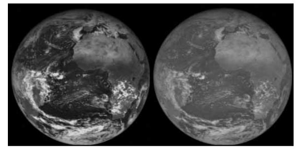
GERB images taken at 12.55 UT on 1 February 2003. The one on the left shows radiances in the short- wave channel, and the one on the right radiances in the total channel
