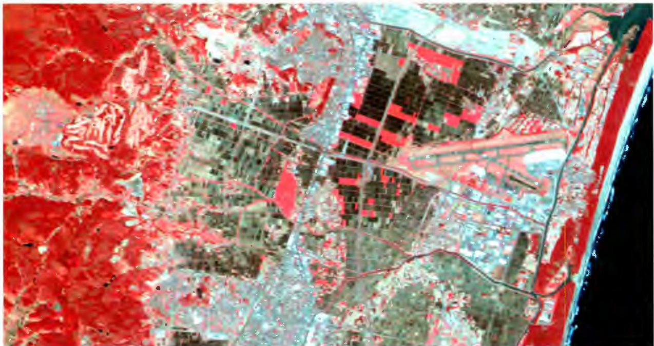
AVNIR-2 images of agricultural land on two separate days. The upper image, made on March 25, 2006, shows cropland planted with wheat in red. The lower image, made on May 4, 2006, was taken in the middle of the rice planting season. The red regions in the center are where rice planting has been completed.
