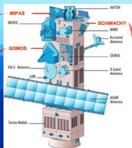
SCIAMACHY Scanning Imaging Absorption spectrometer for Atmospheric Cartography - is a passive remote sensing spectrometer observing backscattered, reflected, transmitted or emitted radiation from the atmosphere and Earth's surface, in the wavelength range between 240 and 1700 nm, and in selected regions between 2000 nm and 2400 nm. The large wavelength range is also ideally suited for the detection of clouds and aerosols.
