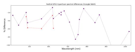
Figure 4-16: Spectral plot of the percentage differences between HyperScan and convolved RadCalNet data.
