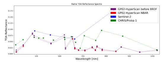
Figure 4-18: Comparison of HyperScan data (with and without BRDF correction) to CHRIS-Proba-1 for Rame Head – marine site.
