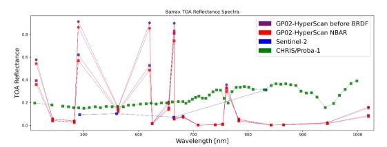
Figure 4-17: Comparison of HyperScan data (with and without BRDF correction) to CHRIS-Proba-1 for Barrax – soil site.
