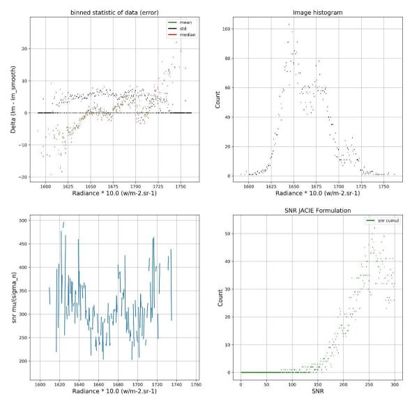
Figure 4-2: SNR plots for the 02 May 2021 band 5 (562.5 nm, green band) in terms of the binned statistics, image histogram and SNR using the simple formula plus cumulative SNR using the adapted formula.
