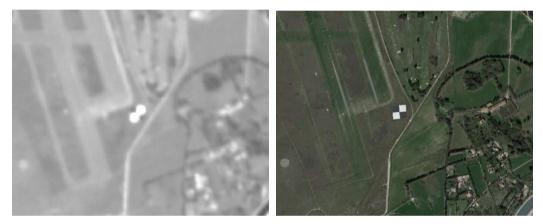
Figure 4-4: Salon-de-Provence MTF target as captured on the 07 April 2021 shown using the 5m resolution panchromatic band (left) and as shown using Google Earth (right) for the same geographical extent.
