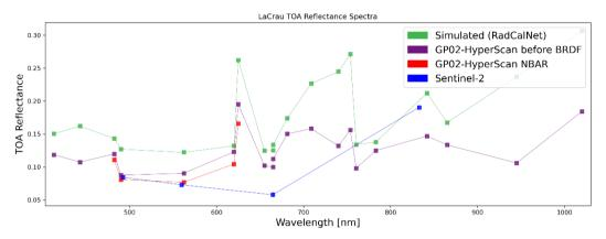
Figure 4-14: Comparison of HyperScan data (with and without BRDF correction, using supplied band convolved solar irradiance data) and RadCalNet convolved to the HyperScan bands.
