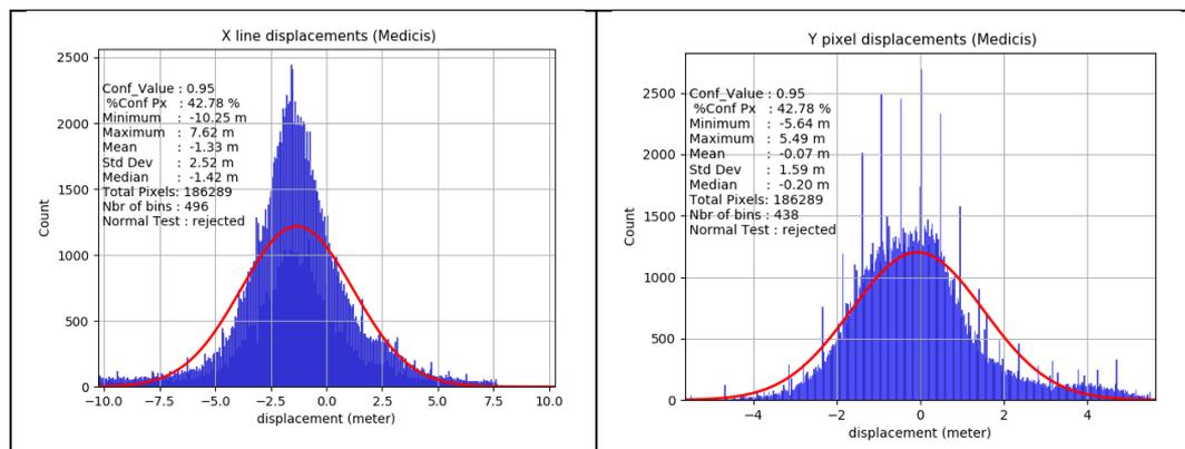
**Figure 5-18: Multi-temporal Geolocation Accuracy – histograms of displacement errors; in line direction (X) / in pixel direction (Y), respectively graphics on the left / right.**
