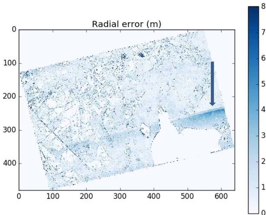
Figure 5-22: Inter-band Geolocation – GREEN / RED Radial error (m).
