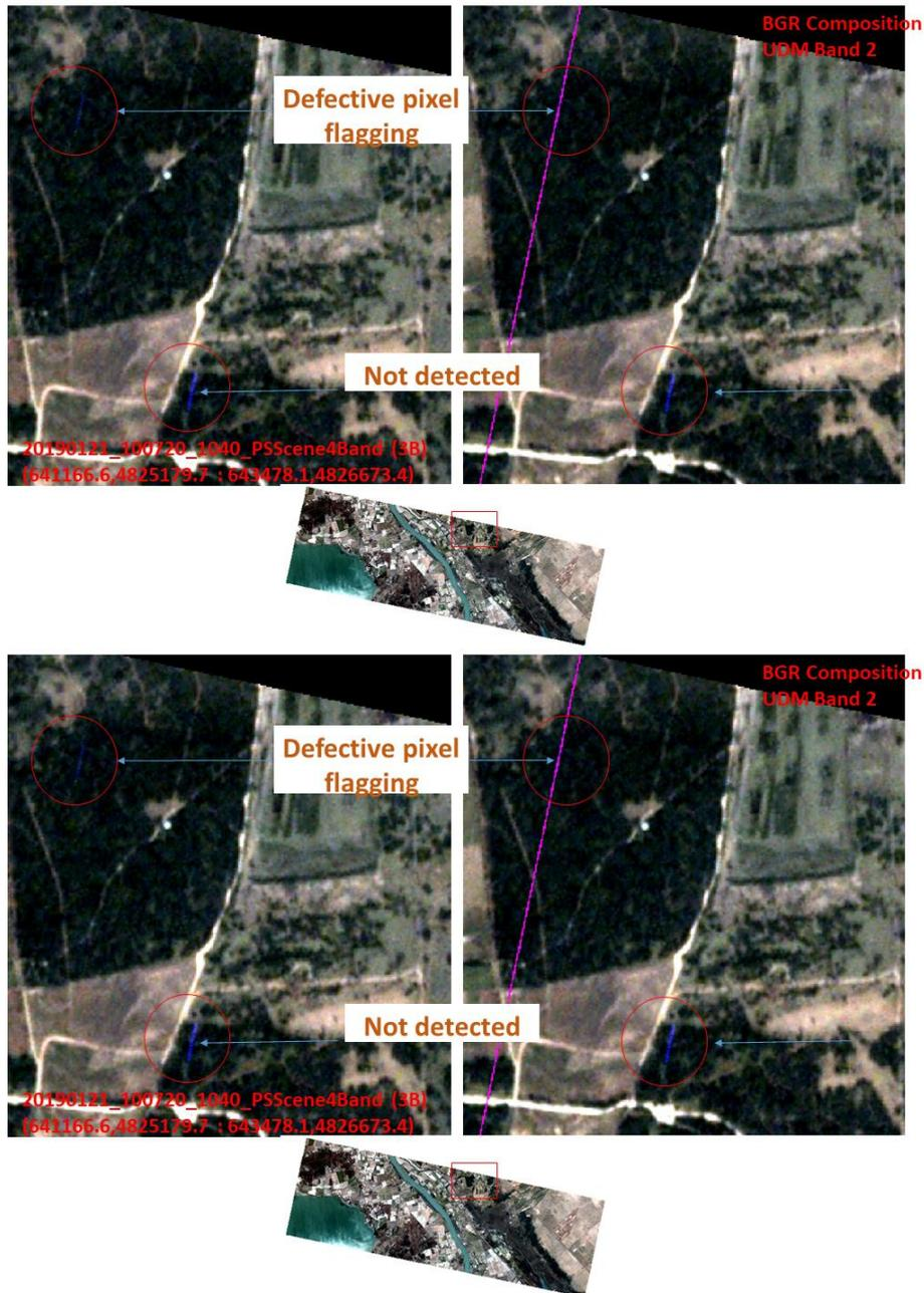
**Figure 5-5: Usable data mask, over detection, false detection, no detection (ID 11).**
