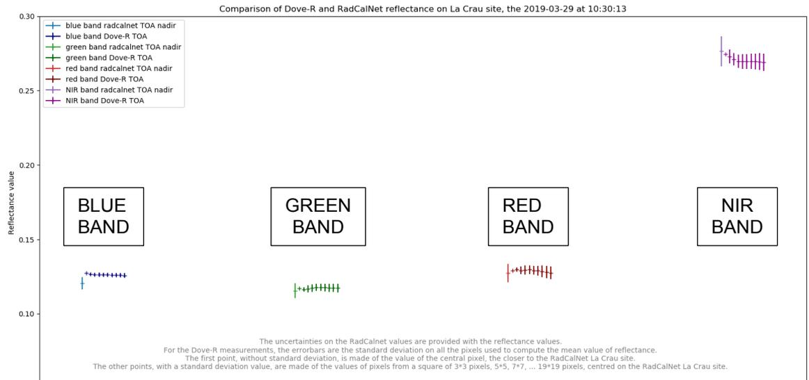
Figure 5-26: DOVE-R TOA Reflectance over RadCalNet LaCrau site, varying the size of the ROI, from one pixel up to 19 x 19 pixels (DOVE-R pixel size).
