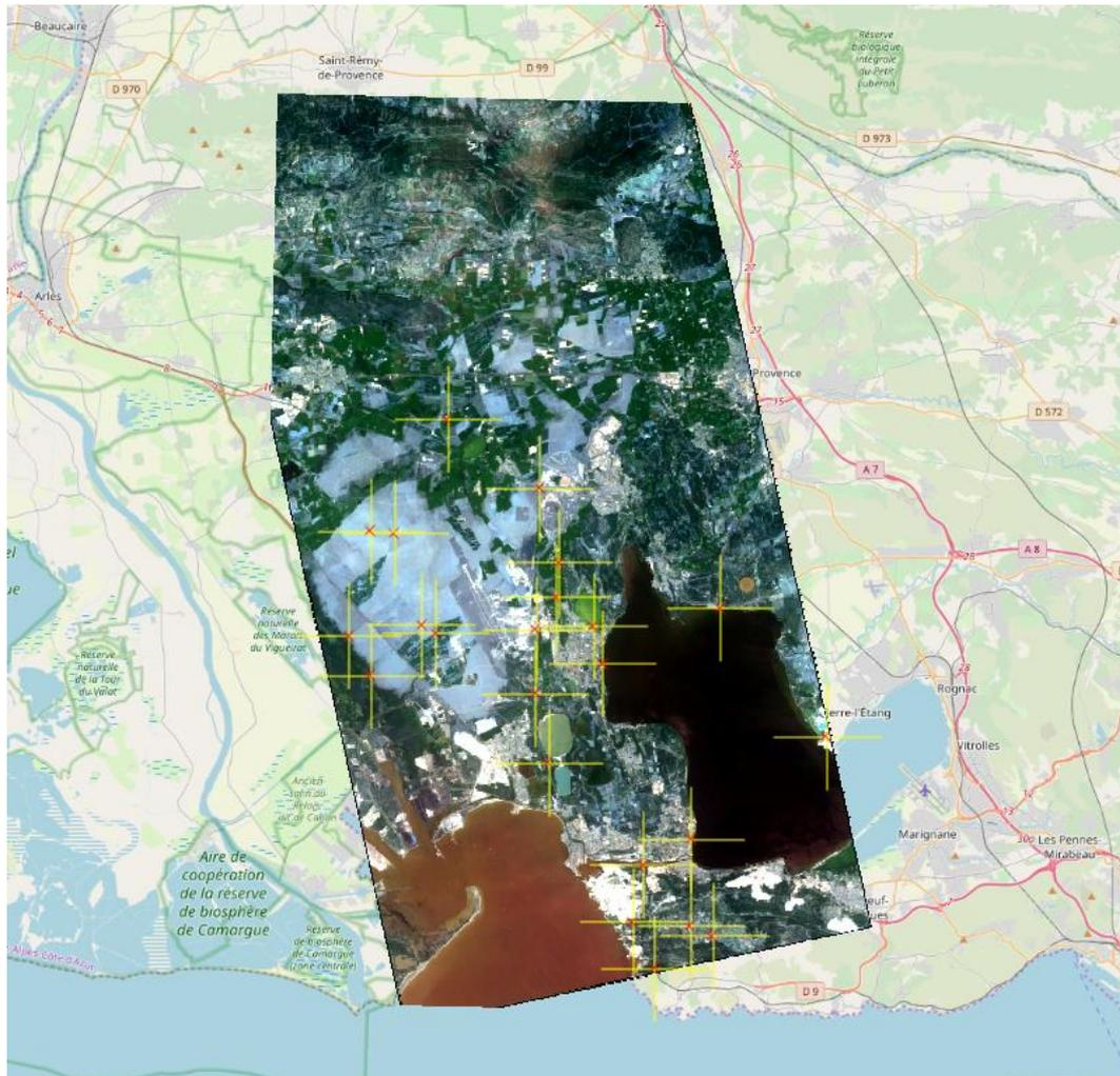
**Figure 5-15: Geometric Accuracy – Composite Level 3A Tile products with Ground Control point set added (La Crau).**
