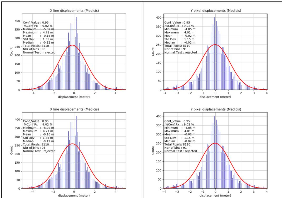
**Figure 5-21: Inter-band Geolocation Accuracy – histograms of displacement errors; in line direction (X) / in pixel direction (Y), respectively graphics on the left / right.**
