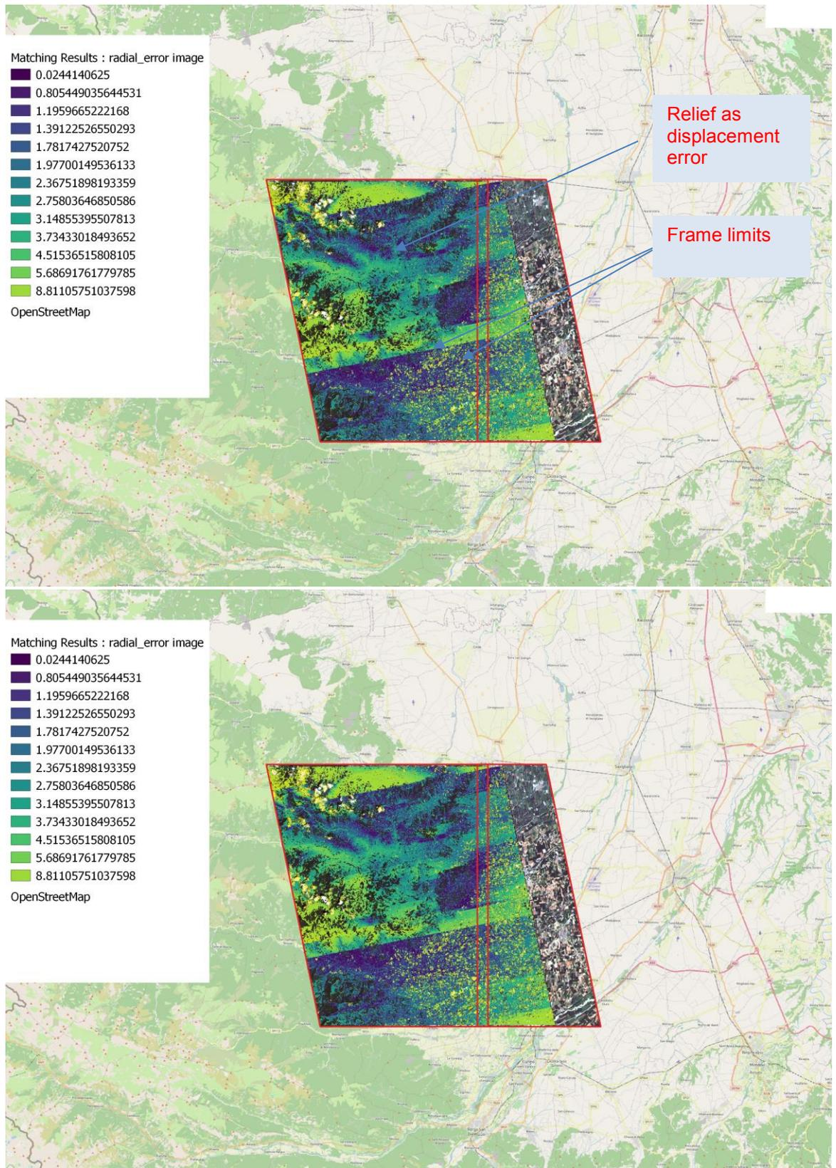
**Figure 5-19: Multi-temporal Geolocation Accuracy - Radial Error Image (pixel) by comparing the two Red spectral band images.**
