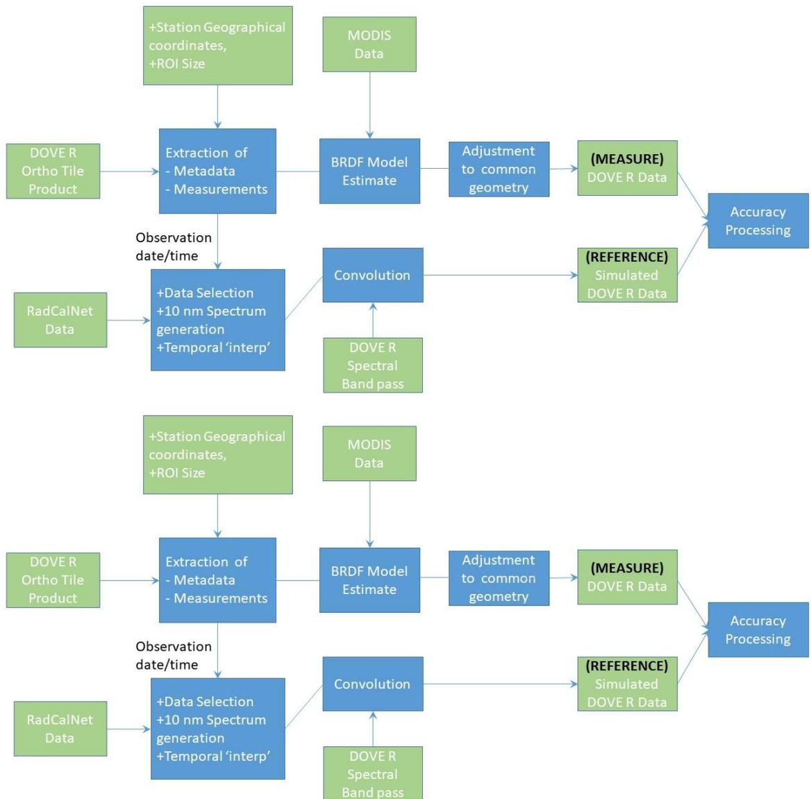
Figure 5-24: The workflow of absolute radiometric calibration using RadCalNet data.
