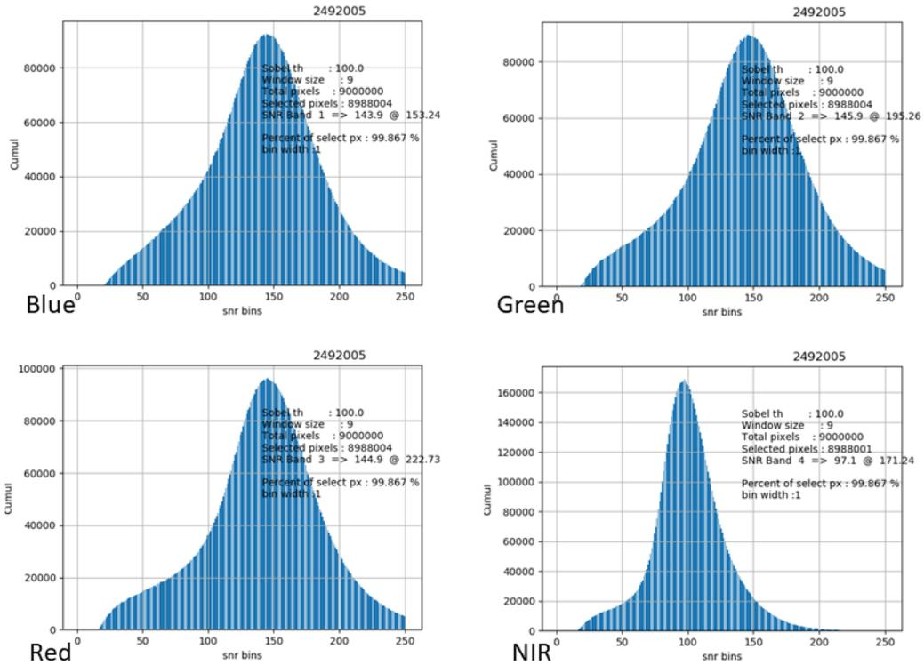
Figure 5-11: The  $\frac{\mu}{\sigma}$ , histogram images for SNR computation.
