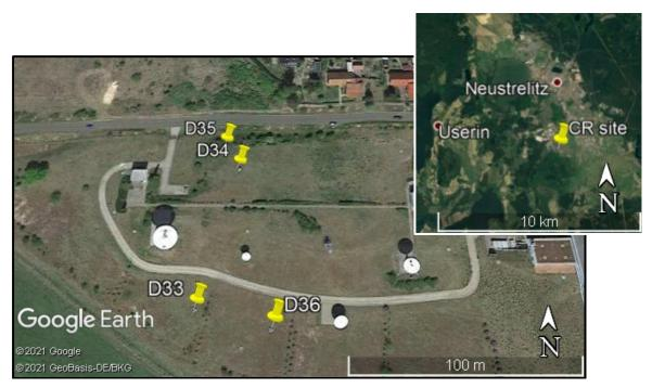
Figure 6: A Google Earth view of the Neustrelitz corner reflector (CR) site in Germany. The small image in the upper right side is a zoom out showing the surrounding area of the CR site. The large image is a zoom in on the CR site, showing the CR names and distribution at the site.
