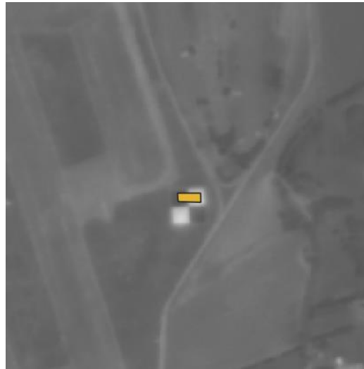
Figure 4-6 Salon-de-Provence Artificial MTF Target: MTF Assessment of NEMO-HD (Panchromatic band only).
