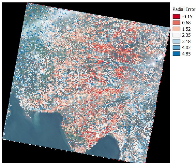
Figure 4-5: The absolute geolocation accuracy result, derived from the image matching tool, using product 5 and reference product.
