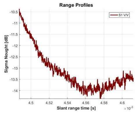
Figure 10: Example of Radiometric Analysis over the Pacific Ocean, expressed in Sigma Nought (dB). Product name: ICEYE\_X2\_SLC\_SM\_7873\_20190817T235839
