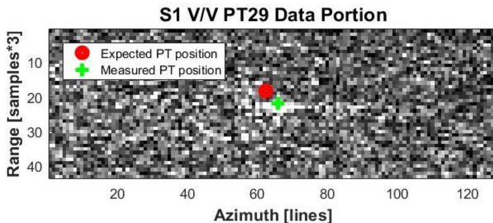
Figure 3. A quicklook image showing the geolocation accuracy of an observed corner reflector.
