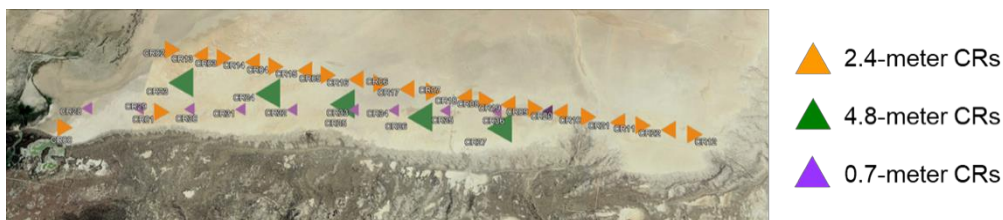
Figure 4 – Corner reflectors exploited for point target acquisitions analyses.
