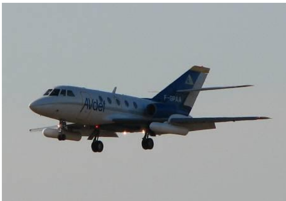
Figure 3-1: The Falcon 20 carrying the SETHI system. The two pods contain the radar antennas.
