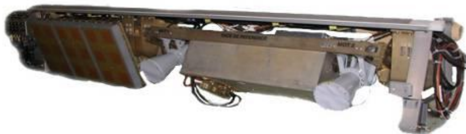
Figure 3-3: The right pod containing the L band antenna and the two X band antennas.
