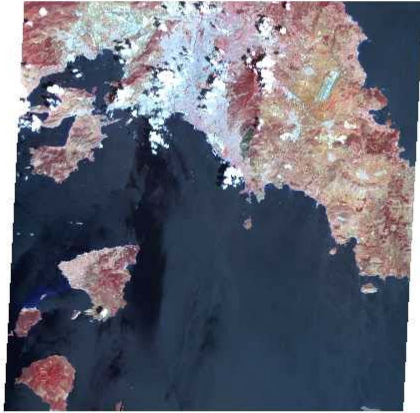
Figure 6. ASTER imagery acquired during over Athens on July 16th (09:22 UTC), during the THERMOPOLIS campaign. This is a false colour composite image produced from the raw visible and near infrared channels of the sensor (R3G2B1). The sensor records information in 15 spectral channels whereas its spatial resolution varies from 15 m (visible to near infrared channels) to 30 m (shortwave infrared channels) and 90 m (thermal infrared channels).
