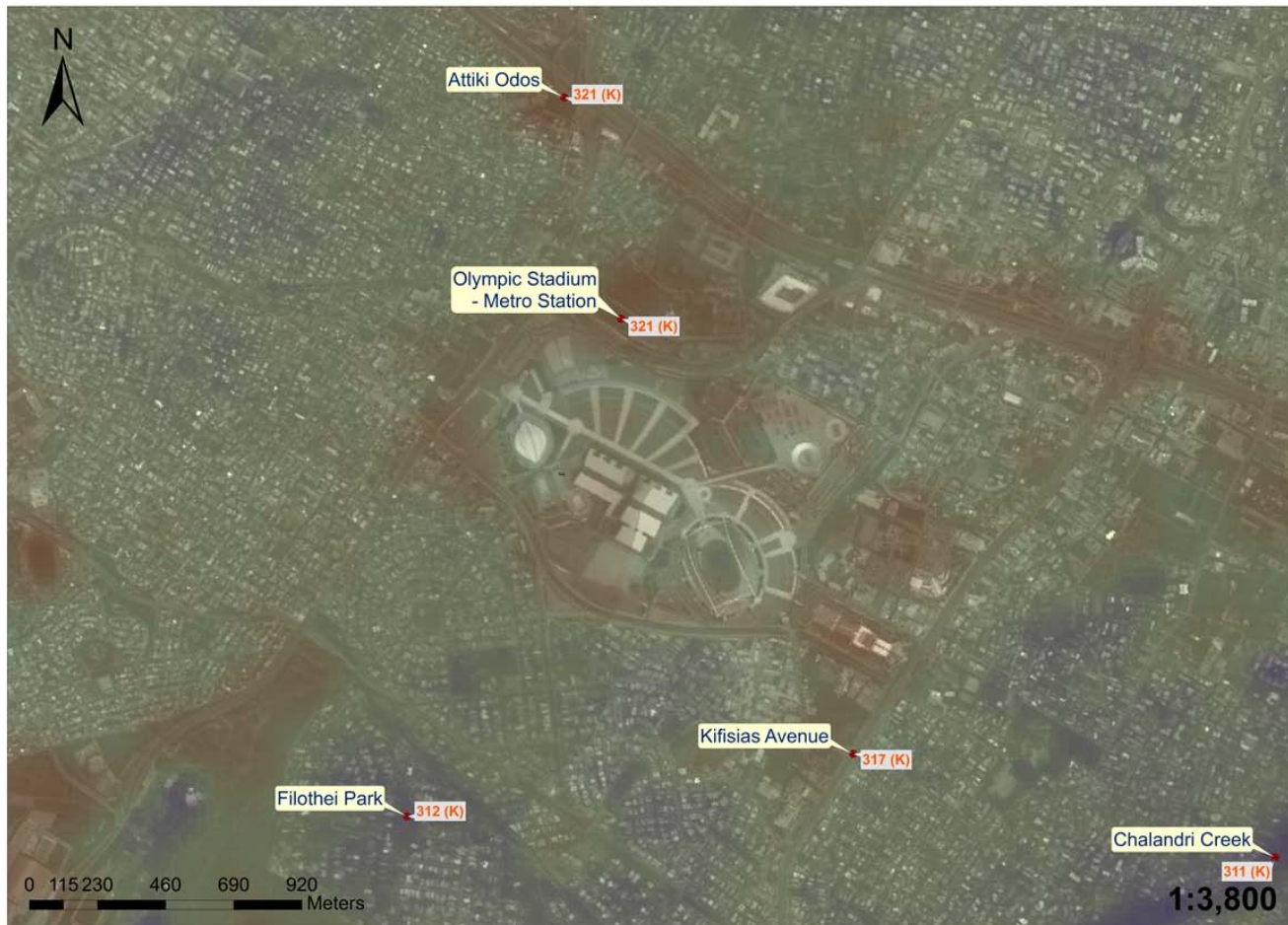
Figure 30: The thermal distribution at and around a complex sports centre. Thermal information is derived from a Landsat image of the morning of 24.07.2009.
