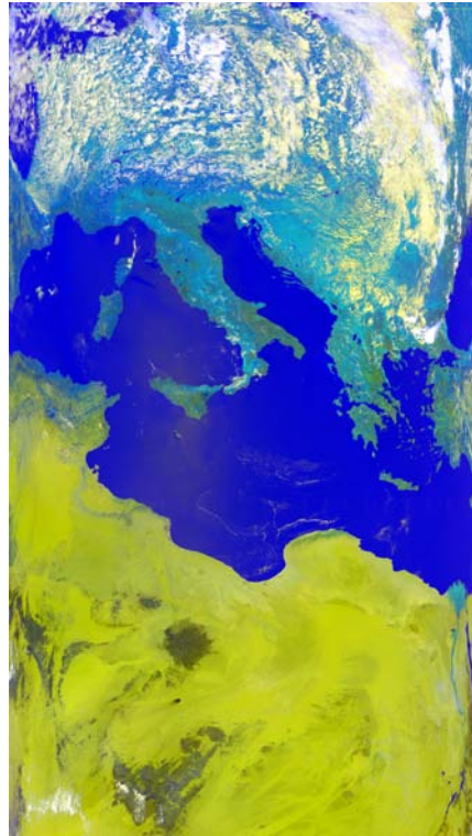
Figure 12. NOAA-19 AVHRR imagery acquired on July 19th (12:10 UTC) over Athens during the THERMOPOLIS expedition. NOAA-19 imagery during the period of the campaign was acquired in real time from the NOA/ISARS receiving station. AVHRR has a nominal spatial resolution of 1 km and it records spectral information in 5 bands from the visible to the thermal infrared parts of the electromagnetic spectrum.
