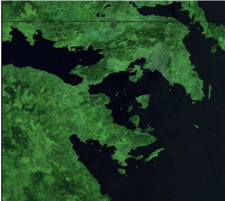
Figure 5. LANDSAT TM imagery acquired on July 24th (08:53 UTC) over the Athens during the THERMOPOLIS campaign. The sensor records information in 7 spectral bands and it has a spatial resolution 30 m in the reflective bands (visible to shortwave infrared) and 120 m in the thermal infrared band.
