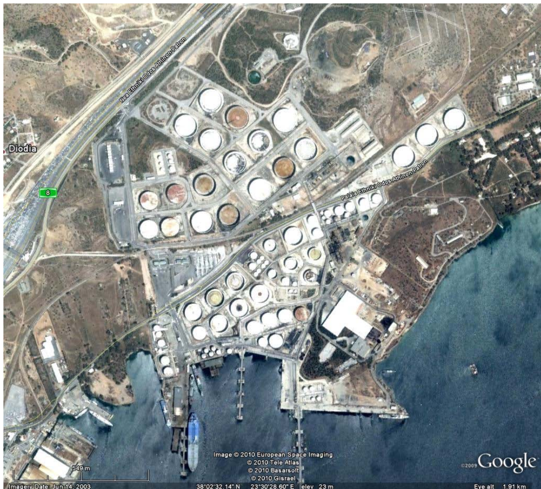
Figure 24: The industrial zone that creates the morning hot-spot of Aspropyrgos and Elefsis (HSM2). It must be noted that the area has (among other industrial activities) refineries consisting of steel tanks. Steel's specific heat is very low ( \sim 500 \text{ J / (kg K)} ) so the area warms up very easily. Steel is also expected to exhibit the small diurnal temperature variations 1 .
