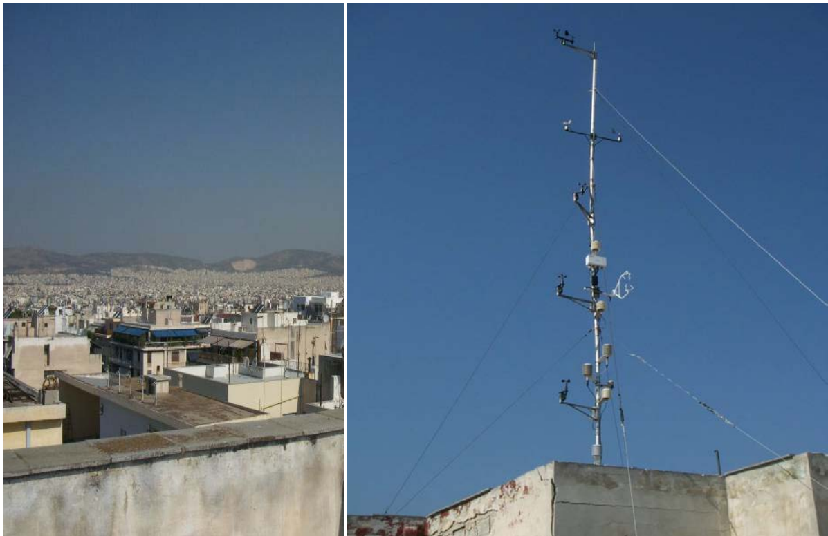
Figure 154. Ten-meter flux tower in the roof of a 7-storey building and the respective fetch.
