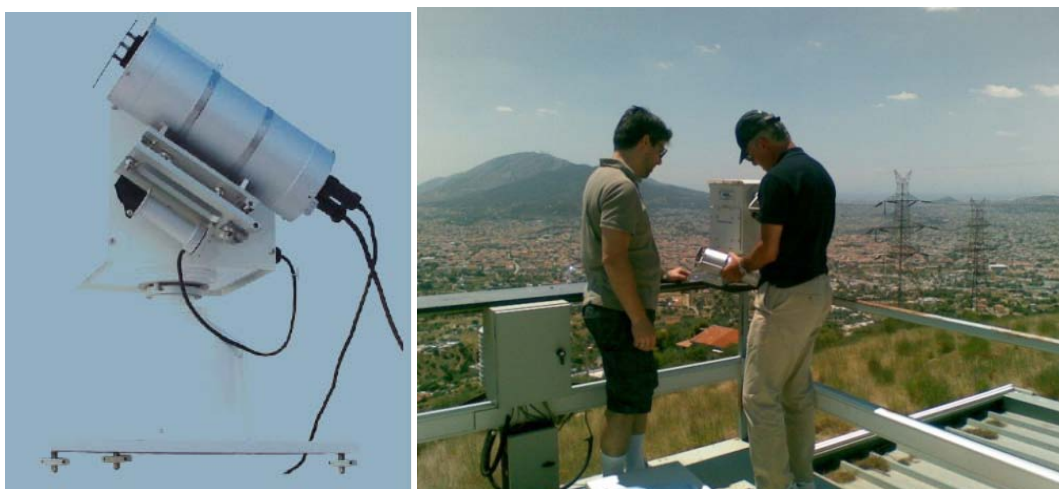
Figure 83: PGS-100 spectrophotometer (left), and the instrument installed at NOA's Penteli station (right)
