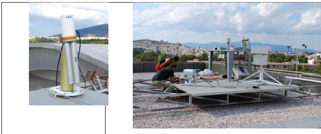
Figure 77. NOA's CIMEL CE318-NEDPS9 sunphotometer and radiometric station in the Academy of Athens site.
