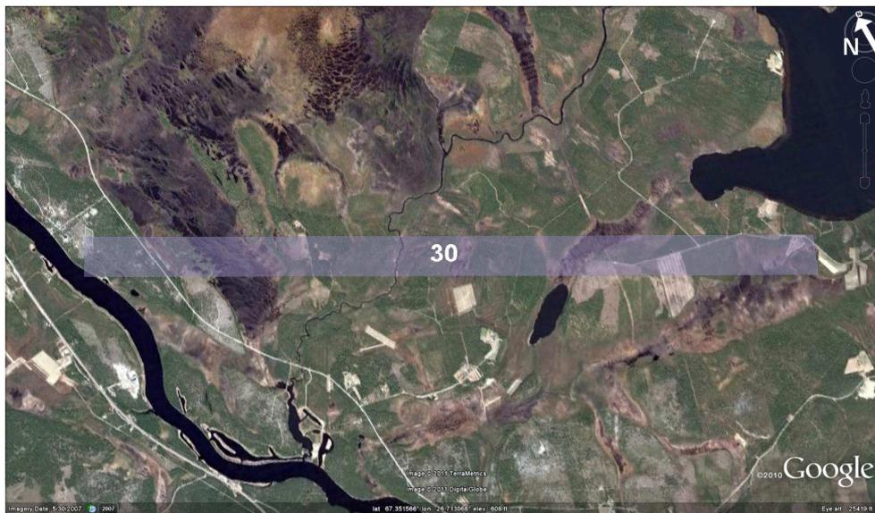
**Figure 16. Ideal ground strip coverage for SnowSAR acquisition flight Nr. 30.**
