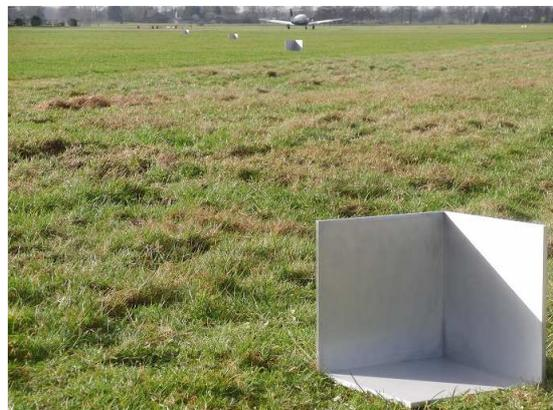
**Fig. 9:** Square-faced trihedral corner reflectors adopted for SnowSAR calibration: deployment during the test measurement campaign of the SnowSAR in Teuge, The Netherlands, February 2011.
