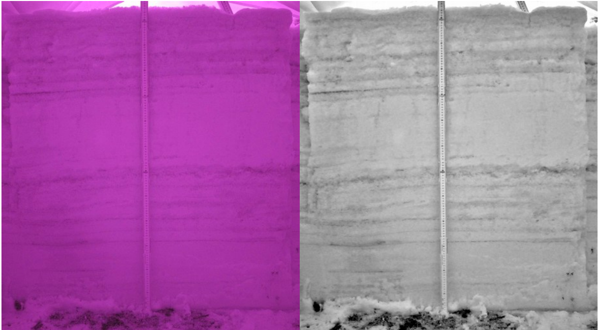
Figure 13 Raw NIR image on the left side and processed image on the right side. The picture shows the snow stratigraphy of the 13. March 2018 on the Davos Laret test site.
