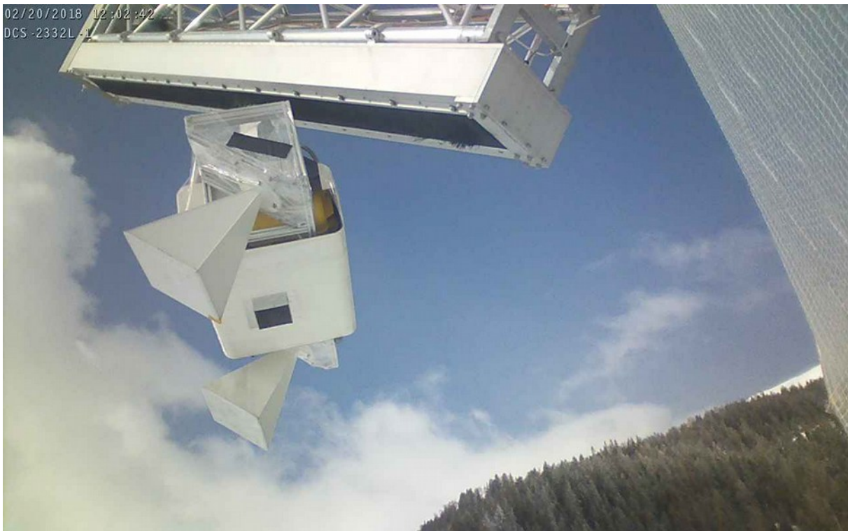
Figure 9: SnowScat is mounted on the tomographic rail that allows a displacement along the rail of about 2.5m. In addition a Quickset pan-tilt-positioner allows to rotate to dedicated angles in elevation and azimuth.
