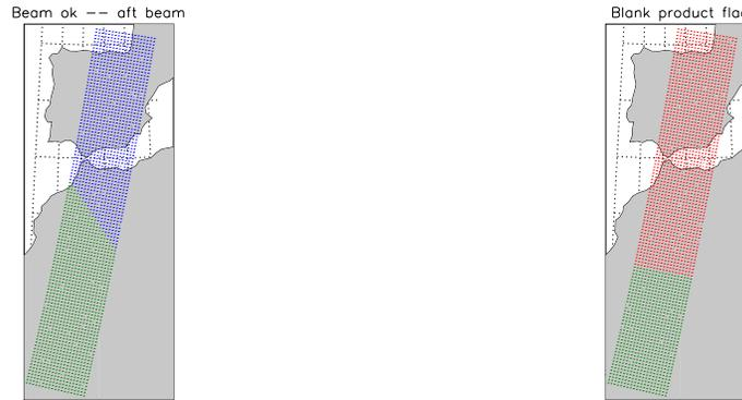
Figure 5.20: Beam ok flag for the Aft (left) beam (green means the flag is set) and blank product flag (right) — red means the flag is set.
