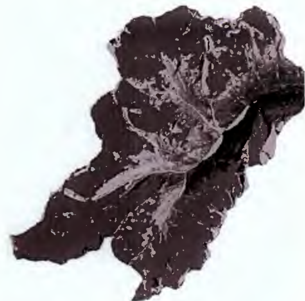
Figure 4-21: Snowcover map of the basin Rofenache on 1 June 1992, derived from ERS-1 SAR data.
