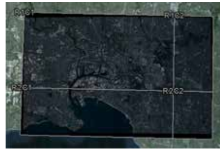
Figure 4.2: Product tiling If a product is not tiled, the file name is: 'product_R1C1.JP2'
