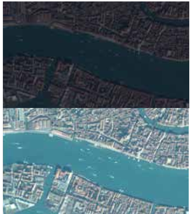
Figure 3.2.2i: Example of an 8-bit product without linear adjustment (top) and with linear adjustment (bottom).
