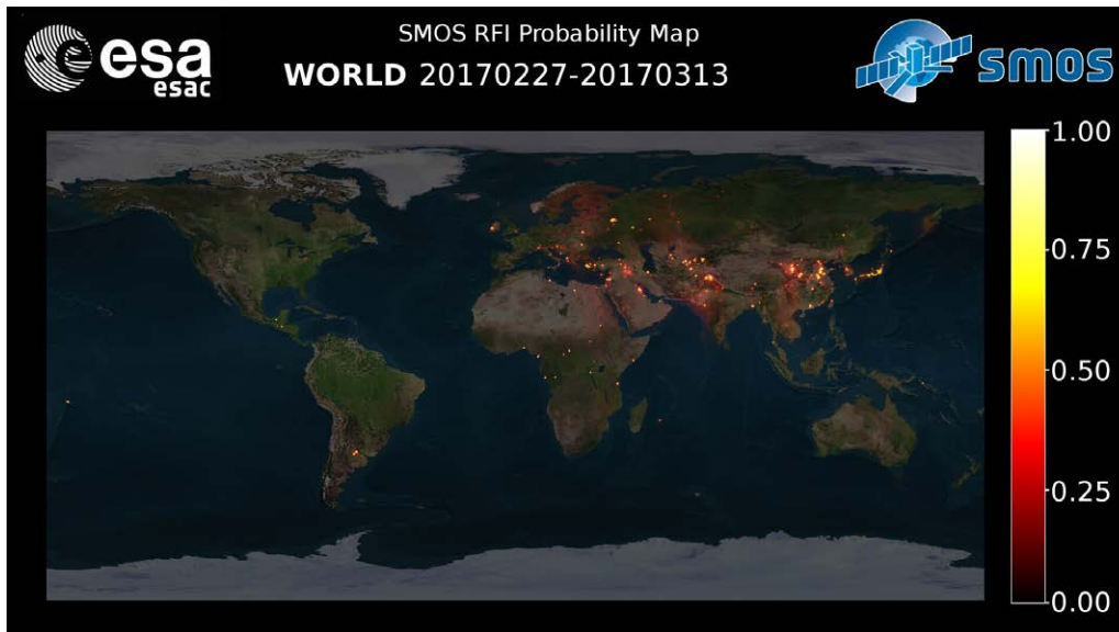
Figure-6: Global map of probability of RFI occurrences during the period 27 th February to 13 th March 2017. The scale indicates percentage of passes when the RFI was detected in a specific area.
