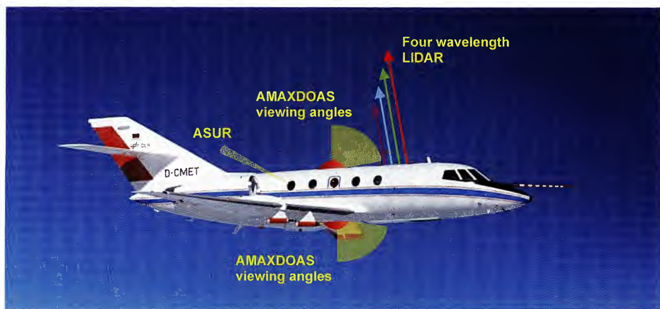
Fig. 9.7 The Falcon aircraft with the viewing directions of the validation instruments (Courtesy: Fix et al. 2005).
