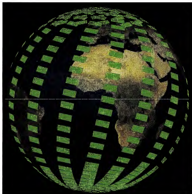
Fig. 4.8 Nadir coverage after 1 day of routine measurements. At the equator consecutive nadir ground pixels are separated by about 1600 km. This gap is filled within 3 days in case of nadir only state sequences. With successive limb/nadir states full nadir coverage at the equator requires 6 days (Courtesy: DLR-IMF/ SRON).
