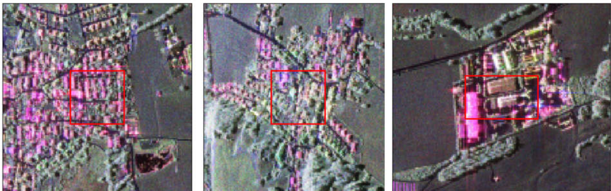
Figure 6.3: Pauli composite images around urban areas which are further analysed. The red rectangle shows the areas which are used for all further evaluations. Left: "Urban 1" (area: 132 m x 120 m), middle: "Urban 2" (area: 132 m x 120 m), right: "Urban 3" (area: 132 m x 210 m).
