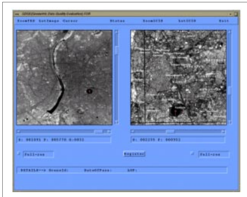
Figure 3.8.2 Screen layout for GCP Id when reference is LISS-III / PAN image with rectified corner coordinates
