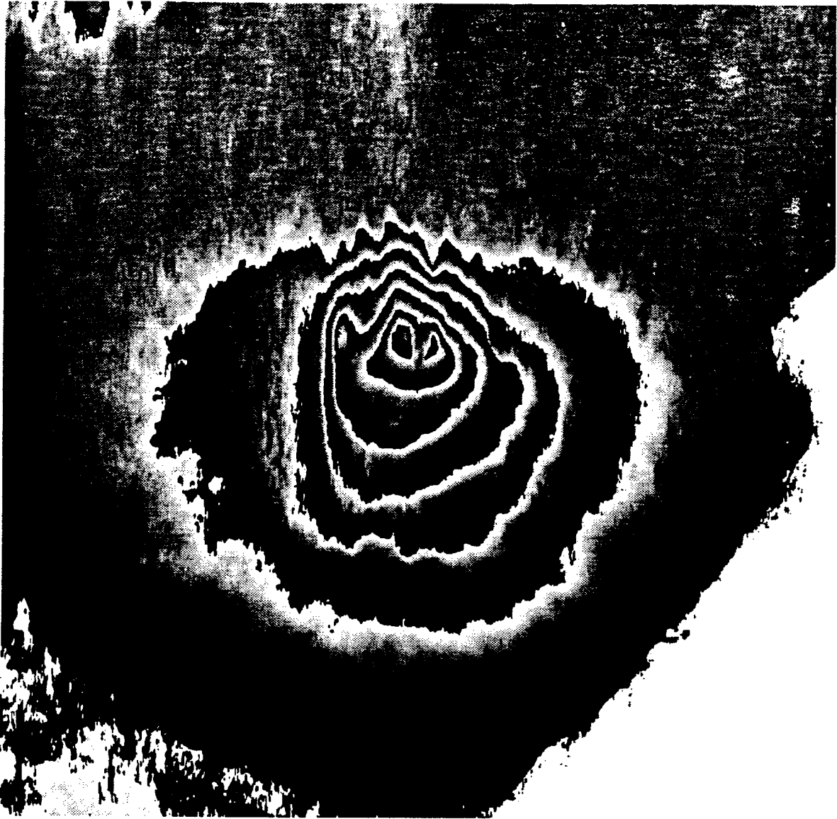
Figure 6.9: ERS-1 interferometry. Unwrapped phase of Mt. Vesuvius presented with a circular gray scale (200meters per cycle). An approximate topography has been reconstructed in correspondence to low coherence regions too (see figure 2.8).
