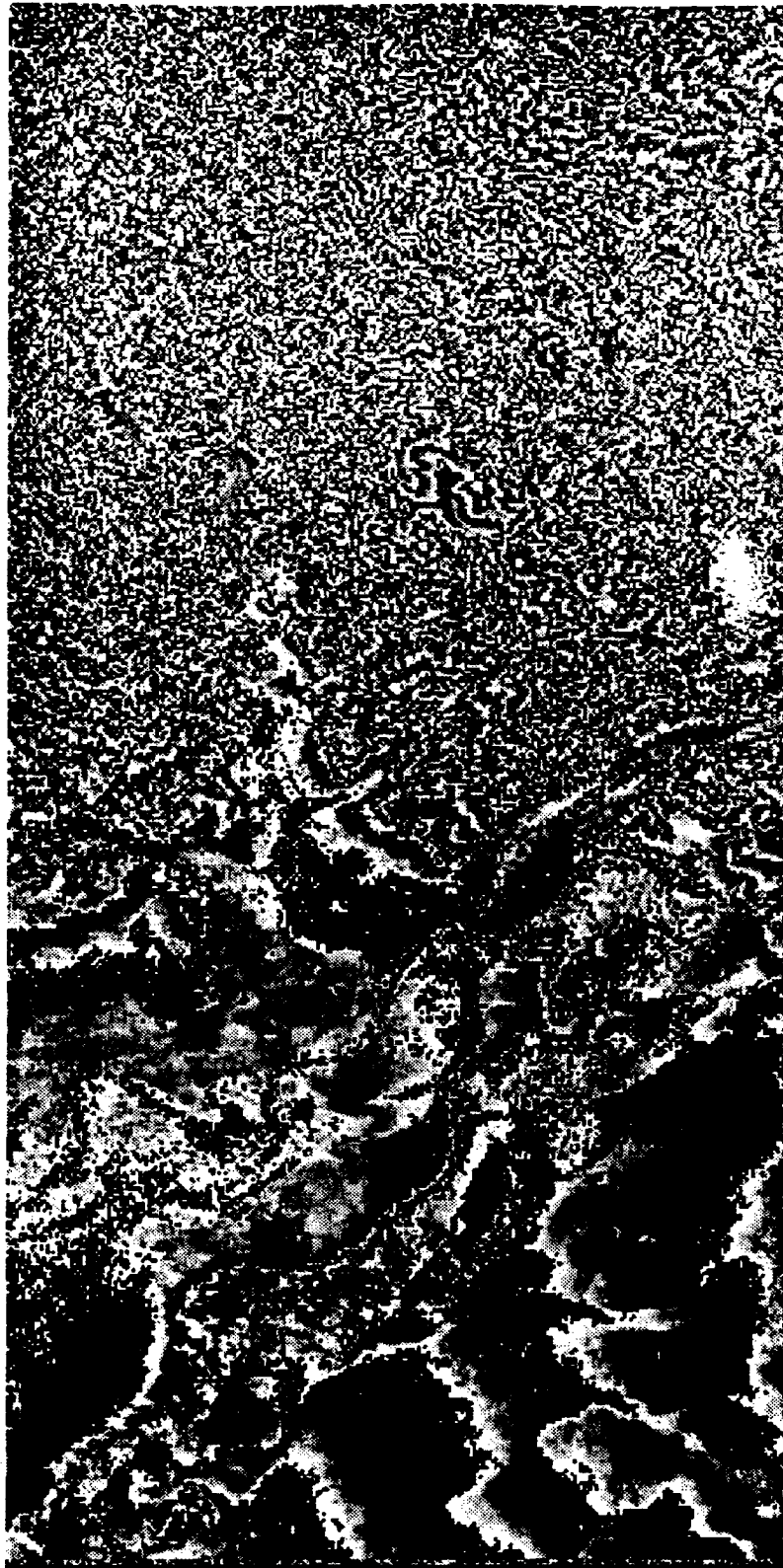
Figure 5.12: ERS-1 SAR interferometric quick-look. Interferometric fringes of Bonn area (Germany). The baseline is about 200 meters.
