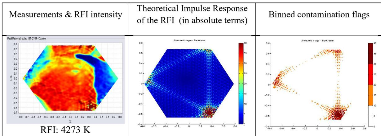
Figure 5: RFI contamination signal characterization process. Left figure shows one SMOS snapshot with presence of one strong RFI. Middle figure shows the estimated impulse response of the RFI signal for the same snapshot. Right figure shows the quantization level in 4 bits of the middle figure.
