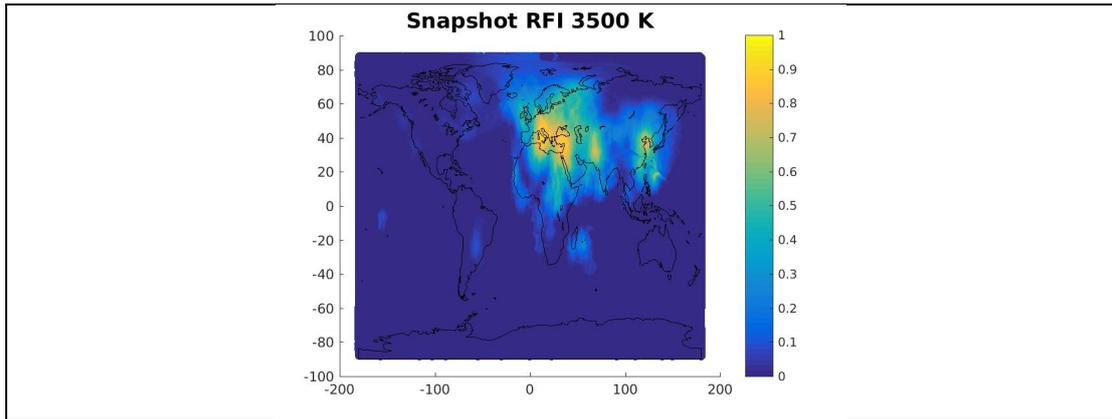
Figure 6: Global map of the occurrence of the snapshot-based RFI flags for a 6 day period in March 2020.
