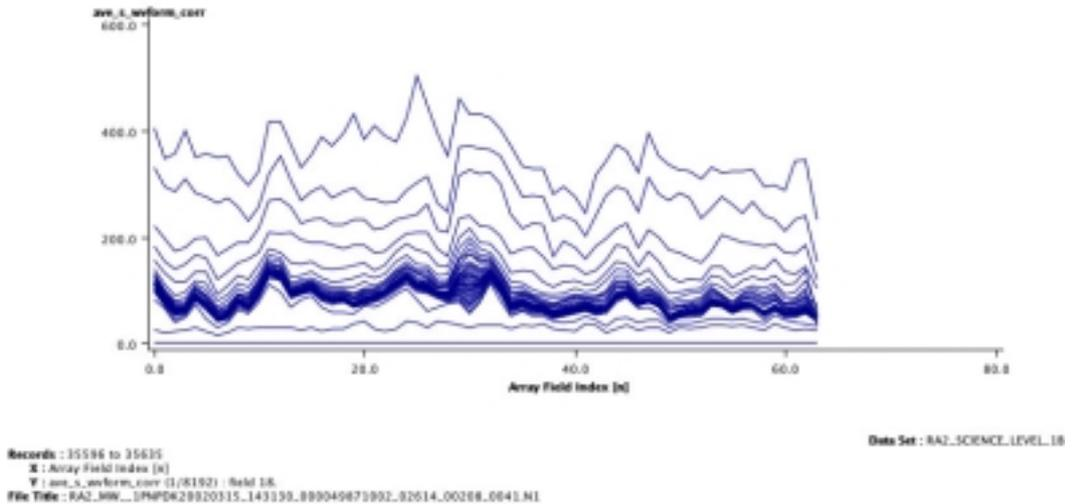
Figure 6. Sequence of 40 S-Band echoes following the acquisition sequence at record 35596. The land echoes are seen to accumulate with the power in each fft sample increasing with each echo received.
