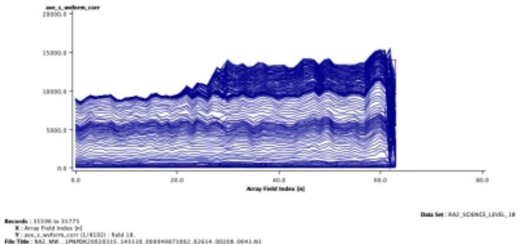
Figure 7. Sequence of 180 S-Band echoes following the acquisition sequence at record 35596. The land echoes are seen to accumulate first with the power in each fft sample increasing with each echo received. Following transition to the ocean the characteristic S-Band ocean echoes are seen to be added on top of the land echoes already received.
