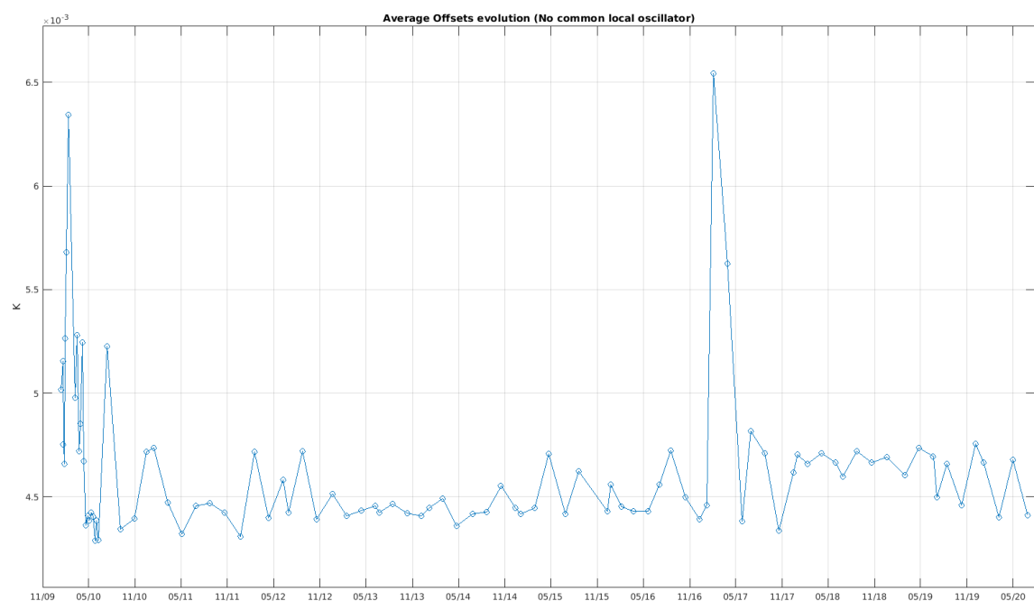
Figure 35 Evolution of the average of the Correlator offsets for the baselines which do not share local oscillator
