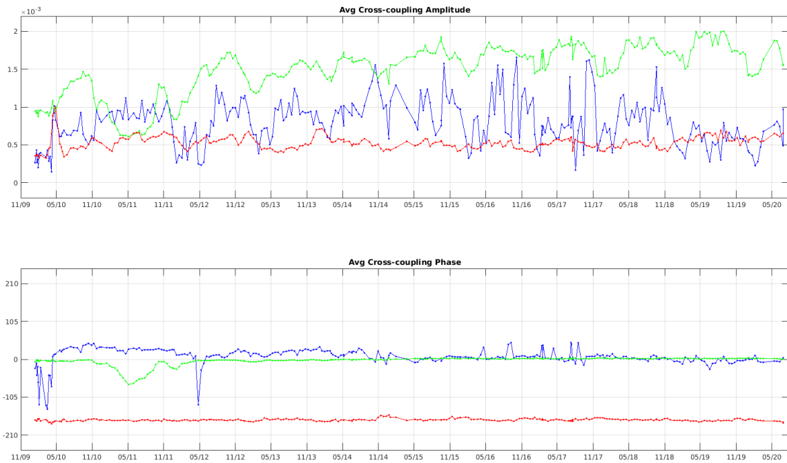
Figure 7 Cross-coupling evolution in amplitude and phase of NIR AB (blue), NIR BC (green) and NIR CA (red) since the beginning of the mission
