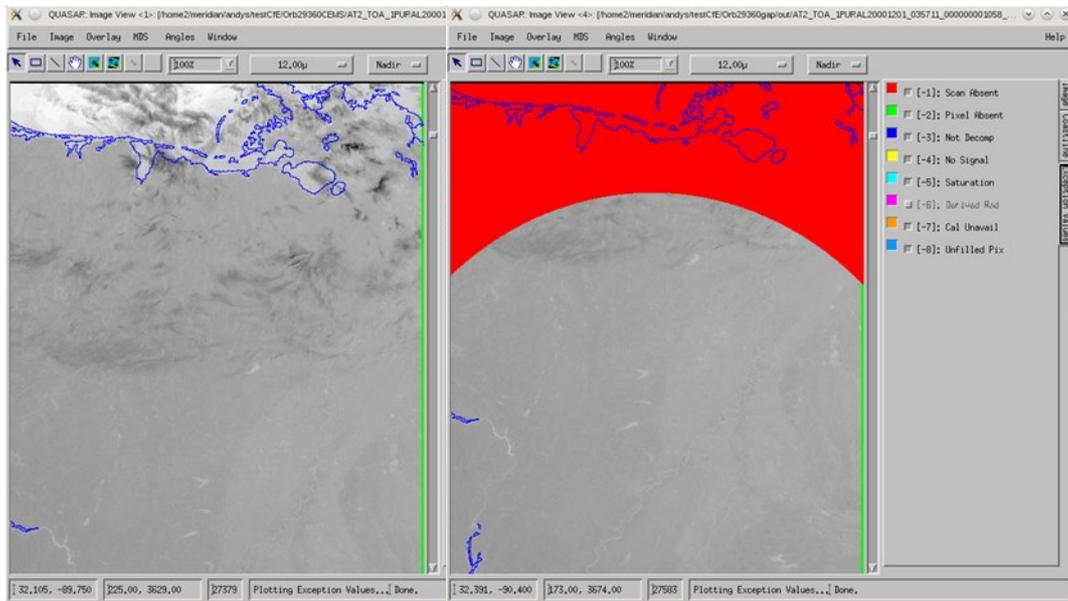
Figure 1: Comparison of two QUASAR screenshots from Level 1B products for the same scene. Left: archived product from the 3<sup>rd</sup> reprocessing. Right: test product with an artificial gap created by removing UBT products from the input.
