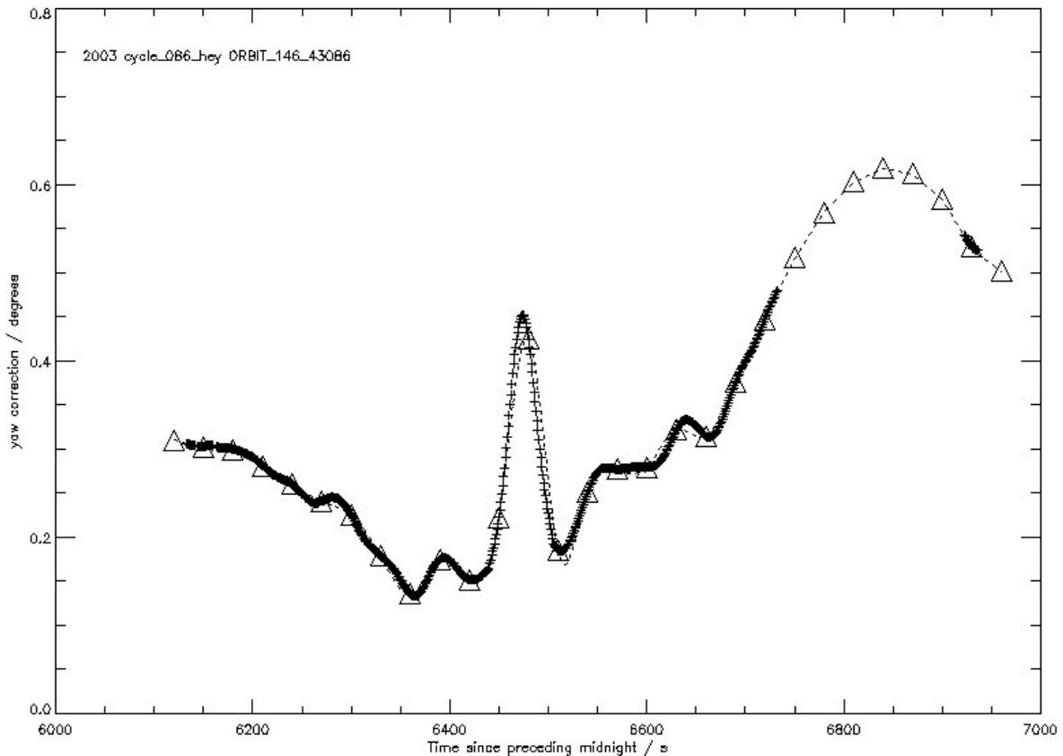
Figure 4: Interpolation and extrapolation of HEY data. Symbols: ++ HEY data,  $\Delta\Delta$  HEY “stack” (spline fit, 30s samples), -- HEY data (reconstructed from stack). Each end of the curve is extended (to the next sample point) by “external” extrapolation using a linear fit to the last 10 data points. The large gap towards the right-hand side is filled by interpolation using the spline fit.
