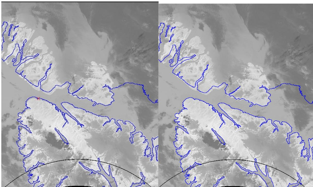
Figure 5: QUASAR screen shot showing a 12µm nadir scene from a Level 1B product processed without HEY data (left) and with HEY data (right). Data from orbit 43098, 18-Jul-2003 21:58:00.
