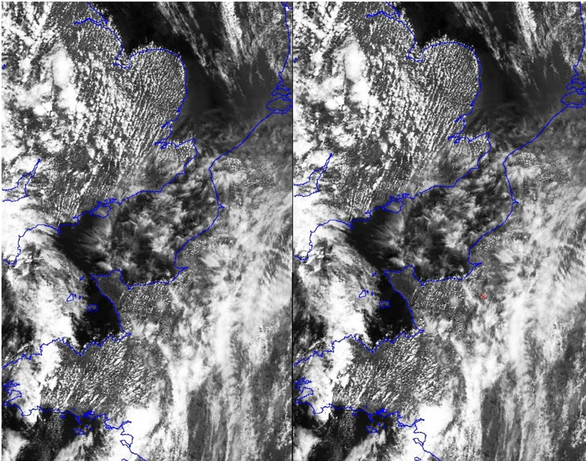
Figure 6: Comparison of 12µm nadir scenes from a Level 1B product processed without HEY data (left) and with HEY data (right). Data from orbit 43120, 20-Jul-2003 10:59:30.
