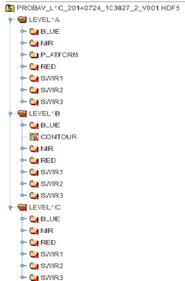
Figure 22: Dataset structure of a segment product file.
