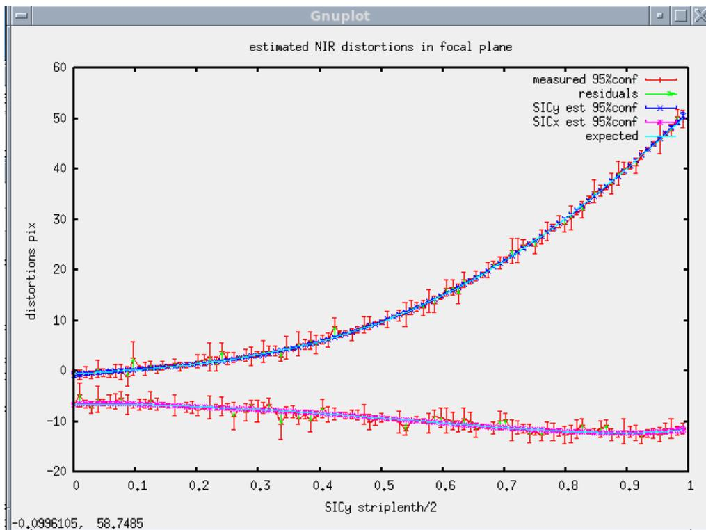
Figure 4.2-15 : example plot of NIR distortion in focal plane
