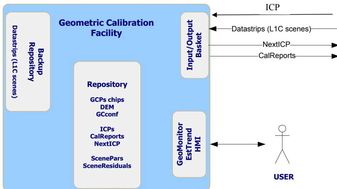
Figure 4.2-4: Geometric Calibration Facility main external and internal interfaces
