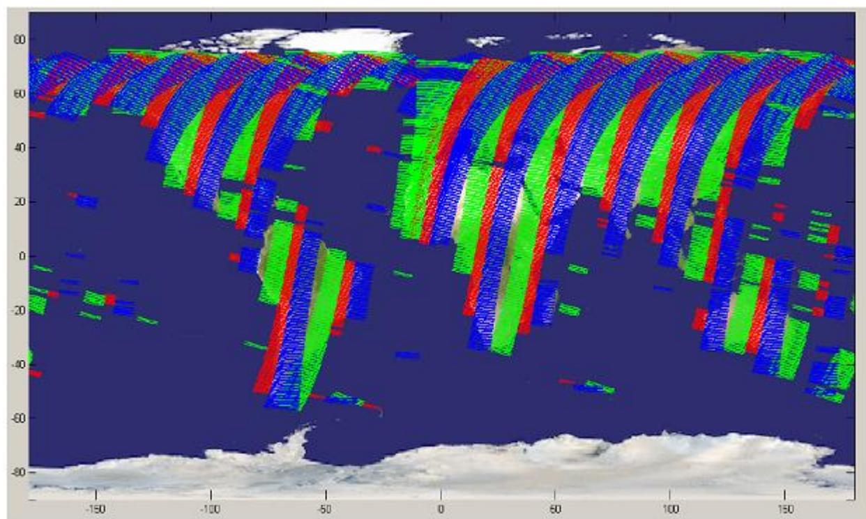
**Figure 4.2 -2: Example of PROBA-V one day coverage of the 3 cameras (1 day orbiting with green=right camera, red= center camera, blue = left camera)**
