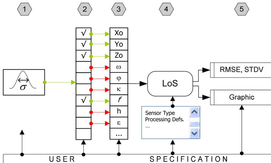
**Figure 4.2-13: Flow chart of sensitivity analysis tool (the green arrows show a possible selected configuration; the red ones possible selections)**
