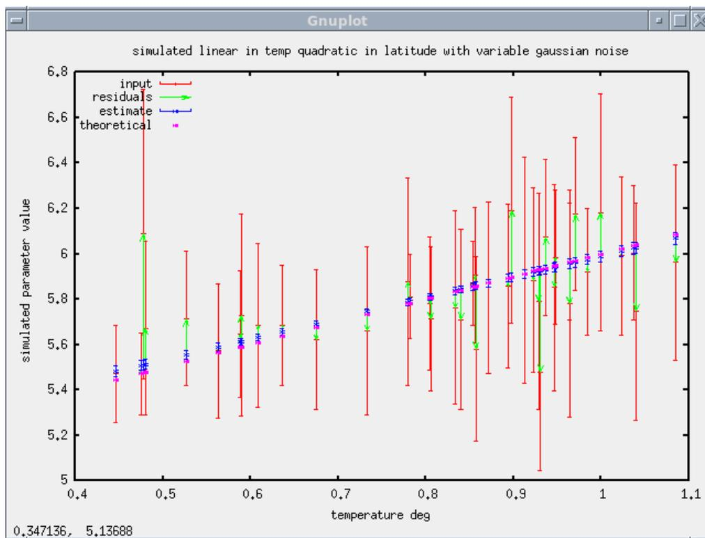
Figure 4.2-14 : example plot of a calibration parameter with 95% confidence against temperature.
