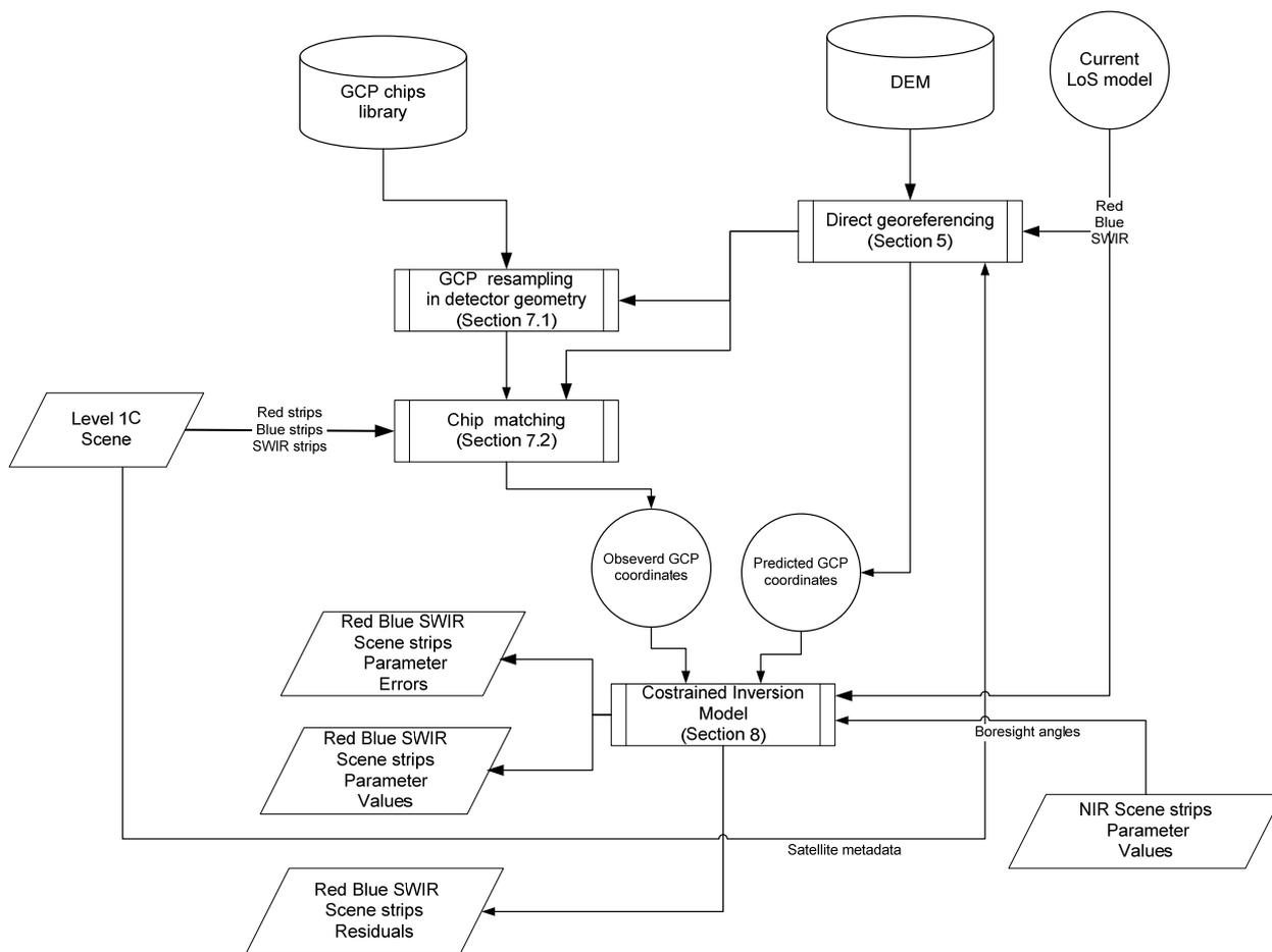
**Figure 4.1-4: Red-Blue-SWIR scene calibration (performed after NIR band calibration)**
