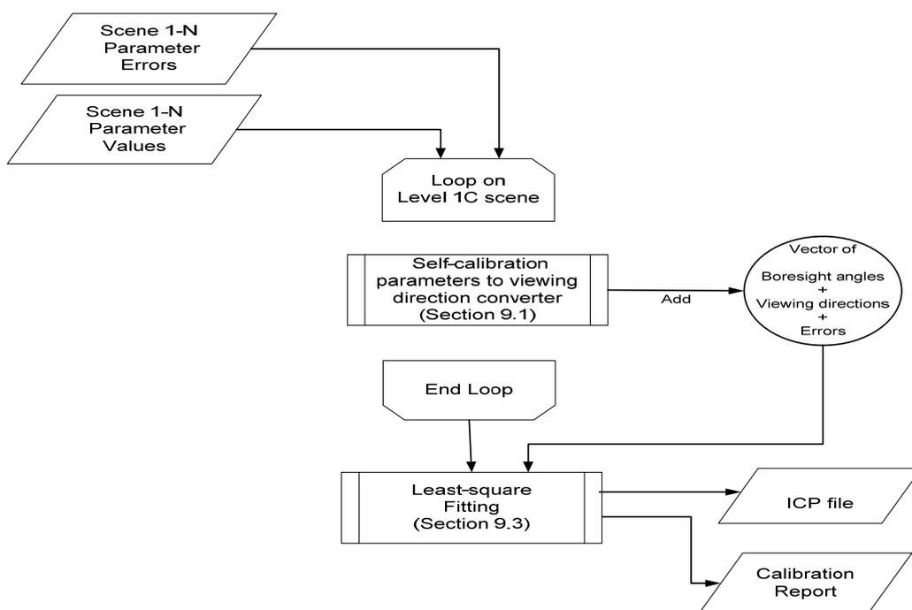
**Figure 4.1-5: Temperature variation Calibration and ICP file generation. In this diagram Interior Orientation parameters (principal point offsets, and polynomial CCD distortions) are called Self-Calibration parameters**
