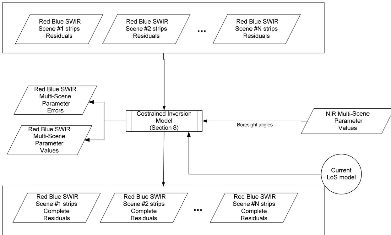
**Figure 4.1-8: Red-Blue-SWIR global-level geometric calibration (performed after NIR band calibration)**
