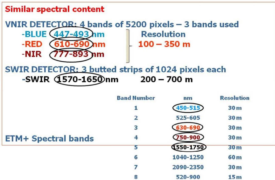
**Figure 4.1-1: Rationale of the PROBA-V/Landsat Geocover bands selection for the geometric calibration. Details are given in Section “GCP Chips Generation”.**
