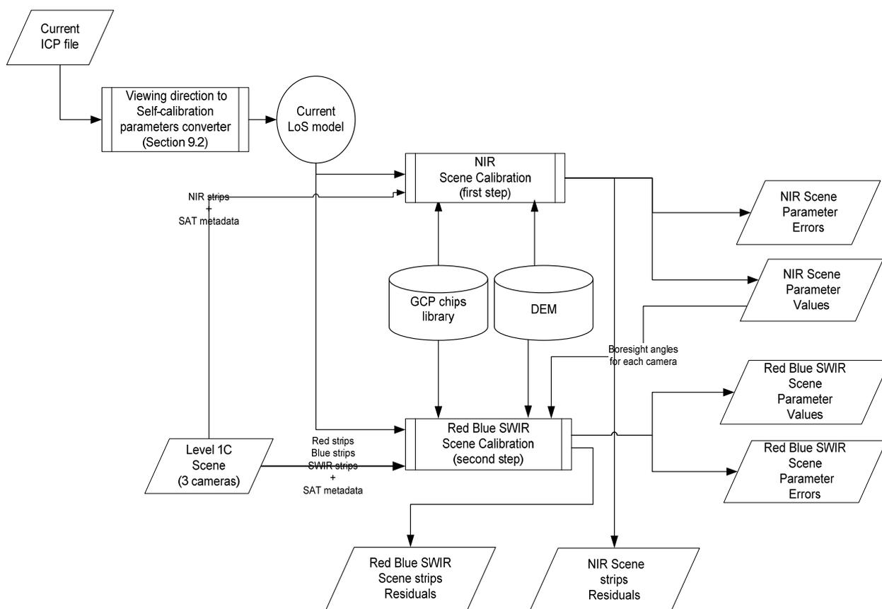
**Figure 4.1-2: Scene Calibration composed by NIR scene calibration and Red-Blue-SWIR scene calibration**
