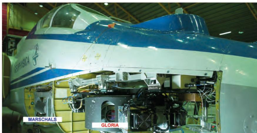
Figure 5.9. The GLORIA imaging FTS and the MARSCHALS millimetre-wave radiometer as accommodated inside the Geophysica aircraft.
