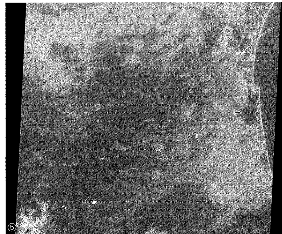
Top-of-the-atmosphere colour composite produced from bands 3, 2 and 1 data of Landsat-5 TM, acquired at Fucino on 1 July 1994.
