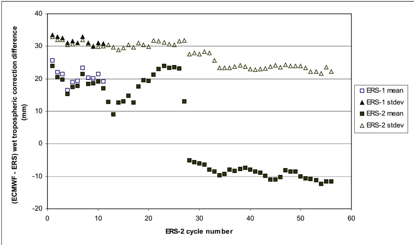
Figure 12 - Mean and standard deviation of the (ECMWF model – ERS radiometer) wet tropospheric correction difference, as function of the ERS-2 cycle number
