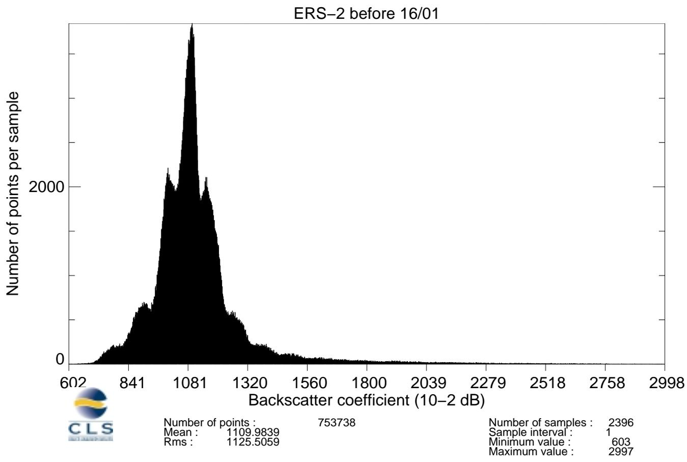
Figure 1 - Histogram of the ERS-2 OPR backscatter coefficient before January 16, 2000
