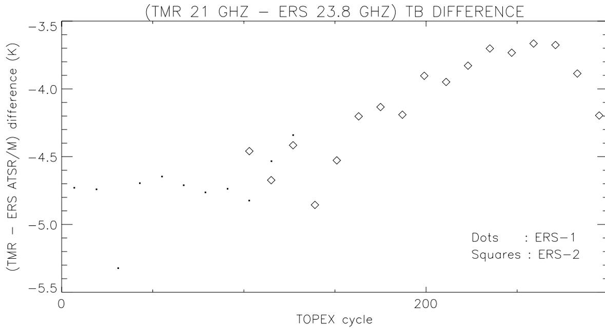
Figure 16 - Mean of the (TMR 21 GHz – ERS 23.8 GHz) brightness temperature difference, as function of the TP cycle. Each dot is a mean over 12 TP cycles.
