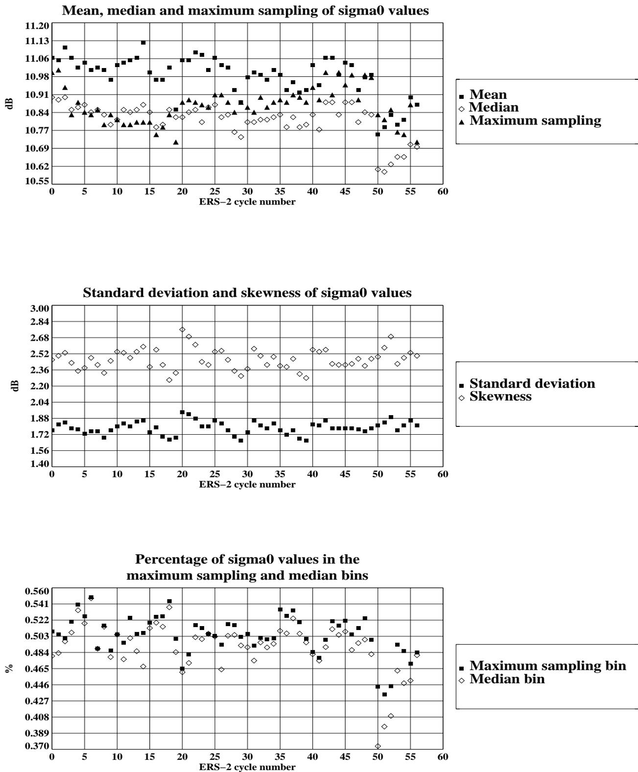
Figure 5 - Statistical results on the ERS-2 OPR backscatter coefficient, as function of ERS-2 cycle number
