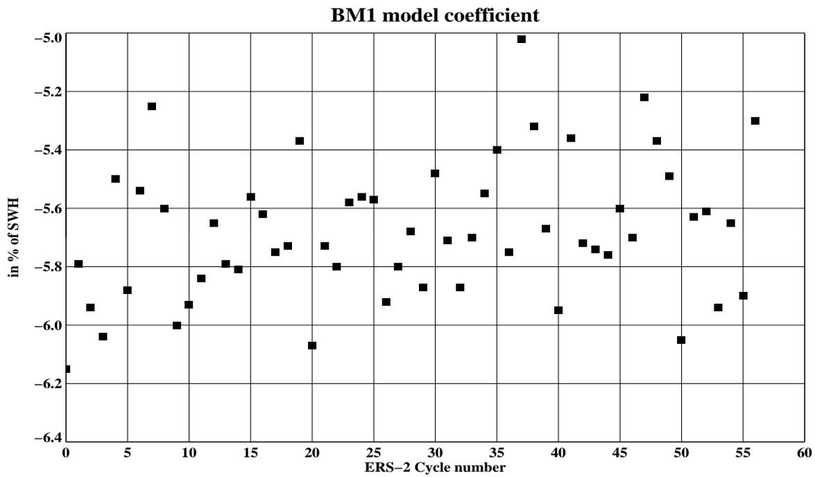
Figure 9 - BM1 sea state bias model coefficient, as function of ERS-2 cycle number
