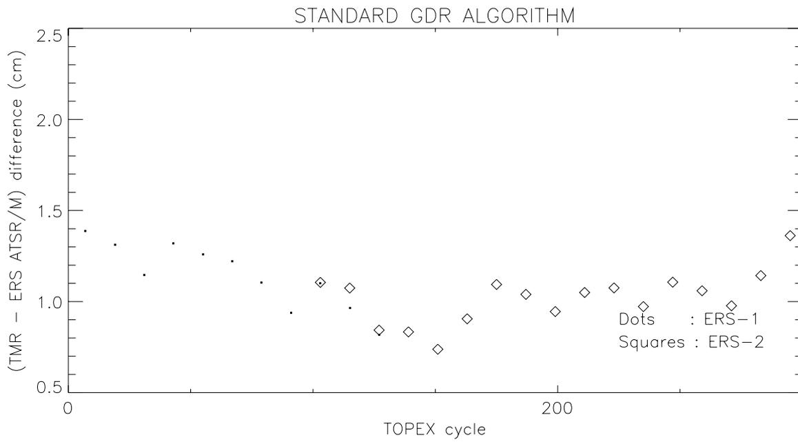
Figure 13 - Mean of the (TOPEX – ERS) radiometer wet tropospheric correction difference, as function of the TOPEX cycle. Each dot is an average over 12 TP cycles.
