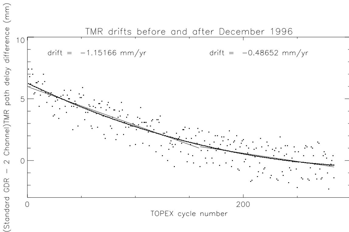
Figure 14 - Mean of the (Standard GDR – two-channel) TMR path delay difference, as function of the TP cycle number. The two channel TMR path delay is computed without the 18 GHz brightness temperature. Each dot is the cycle mean of the difference. Superimposed are a cubic regression fit, and two linear regression lines before and after December 1996. The corresponding drift rates are given on top of the plot.
