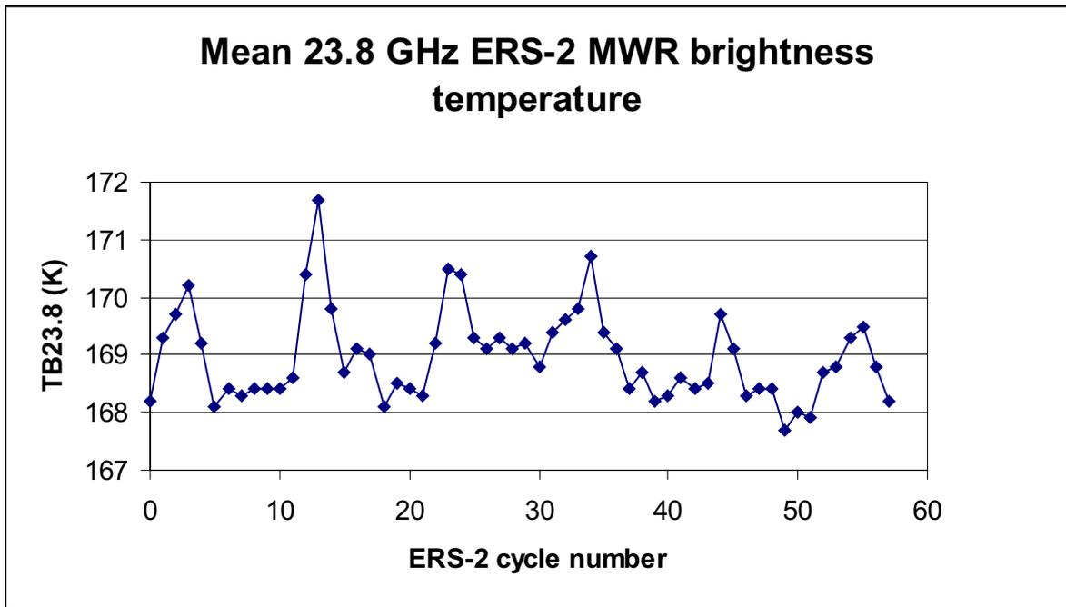
Figure 17 - Cycle mean of the ERS-2 radiometer 23.8 GHz brightness temperature, as function of the ERS-2 cycle number.
