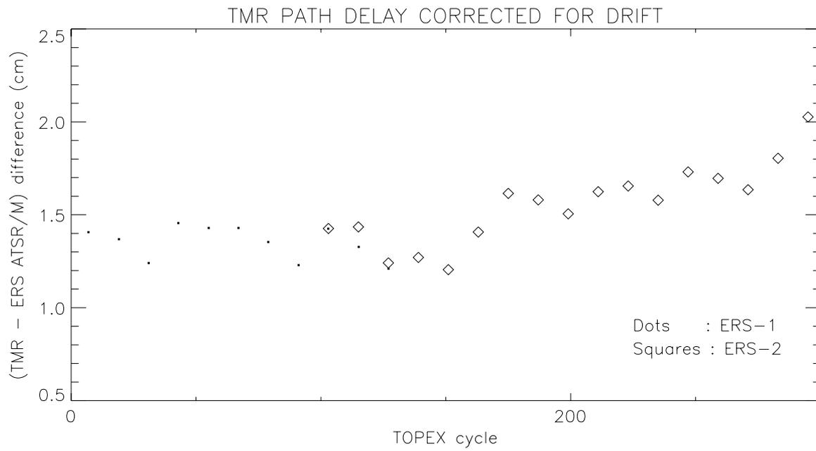
Figure 15 - Same as figure 13 excepted the TMR path delay is corrected for the drift rates given in figure 14.
