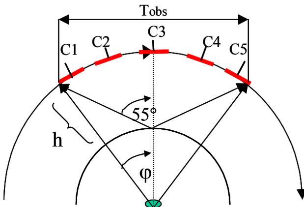
Fig1: Illustration of acquisition geometry. The red lines indicate image acquisitions and  $C1$  to  $C5$  the image centre times. **N.B.  $C1$  and  $C5$  do not correspond to the start and end of the observation time.**
