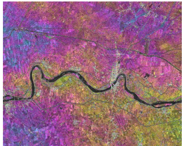
Figure 2 Po Valley, Italy. Combined EET cross-interferogram based on EET pairs on 15-Dec-2007 and 6-Oct-2007 with an effective B_{\perp} 360m.
