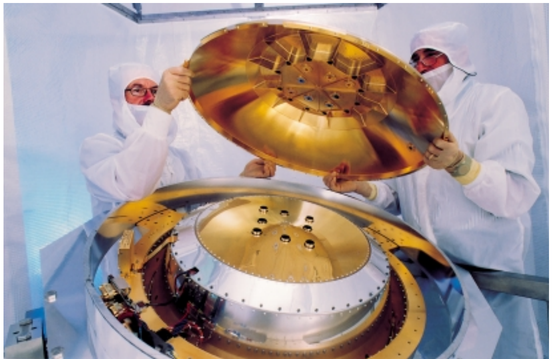
The Radiator Assembly during integration
