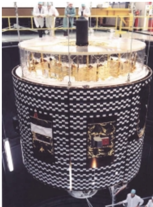
Thermal-balance testing in progress in the Large Space Simulator at ESTEC in Noordwijk (NL)
