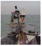
5 August 2003 On measurements seaborne were made for two stations within the Oostende test site. The parameters measured are water-leaving reflectance, SPM and CHL. The water-leaving reflectance is measured by the TriOS instruments (fig. 4). This comprises system 3 which sensors are
