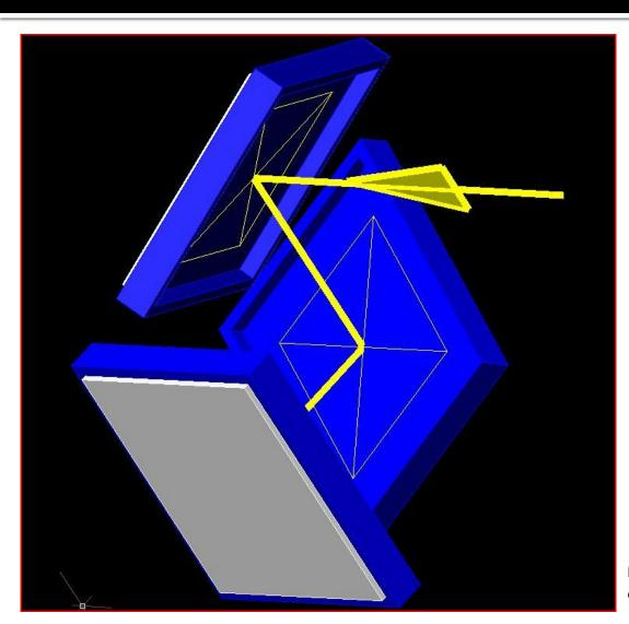
The trap detector consists of three photodiodes arranged in such a way that light can emerge from the detector only after multiple reflections.
