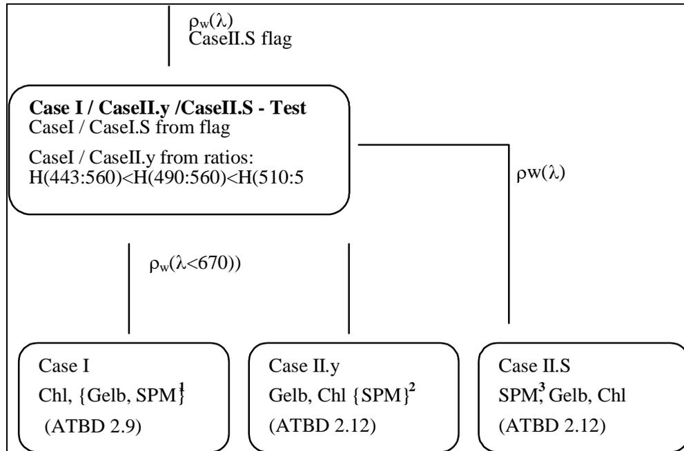
Figure 1 In Water Component of Processing Chain (Bold indicates PML contribution).
