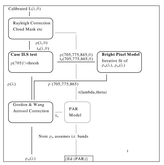
For simplicity in the expression of the iterative method the angles have been compounded into a single term  $\theta = [\theta v, \theta s, \Delta \phi]$ ; the superscript <sup>R</sup> is used to denote values in the LUTs and the superscript <sup>e</sup> is used to denote initial or intermediate estimates.
