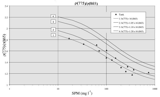
Figure 5 shows the dependence of  $\rho(865)$  on b(SPM) for fixed value a(SPM).= 0.02 m<sup>-1</sup>. The best fit is for b(SPM,865) = 2 m<sup>-1</sup>. This figure although high, matches the fine sediments likely to be in suspension in the majority of shelf seas.
