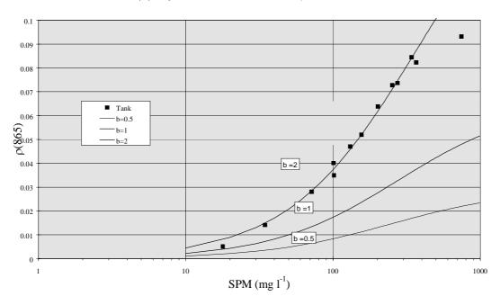
Figure 5.  $\rho(865)$  vs. SPM for theoretical  $\rho(865)$  and a range of b (SPM)
