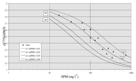
Figure 3 shows the effect of varying a(SPM) on the  $\rho_w(775)/\rho_w(865)$  to SPM relationship. Compared with the effect of b(SPM), the ratio is highly sensitive to small changes of a(SPM) around the test value of 0.02 m<sup>-1</sup>. The a(SPM) = 0.02 m<sup>-1</sup> line fits the observed data best, with the range 0.01 to 0.03 m<sup>-1</sup> bracketing the full data range.
