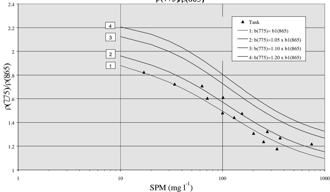
Figure 5 shows the dependence of  $\rho(865)$  on  $b(\text{SPM})$  for fixed value  $a(\text{SPM}) = 0.02 \text{ m}^{-1}$ . The best fit is for  $b(\text{SPM}, 865) = 2 \text{ m}^{-1}$ . This figure although high, matches the fine sediments likely to be in suspension in the majority of shelf seas.
