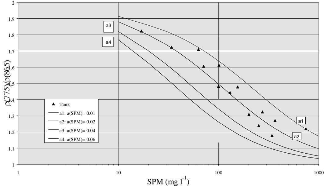
Figure 3 shows the effect of varying  $a(\text{SPM})$  on the  $\rho_w(775)/\rho_w(865)$  to SPM relationship. Compared with the effect of  $b(\text{SPM})$ , the ratio is highly sensitive to small changes of  $a(\text{SPM})$  around the test value of  $0.02 \text{ m}^{-1}$ . The  $a(\text{SPM}) = 0.02 \text{ m}^{-1}$  line fits the observed data best, with the range  $0.01$  to  $0.03 \text{ m}^{-1}$  bracketing the full data range.
