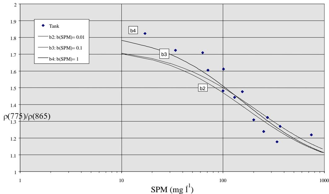
Fig 3.  $\rho(775)/\rho(865)$  vs. SPM for a constant  $b^1(\text{SPM})$  of 0.5 and a range of  $a^1(\text{SPM})$
