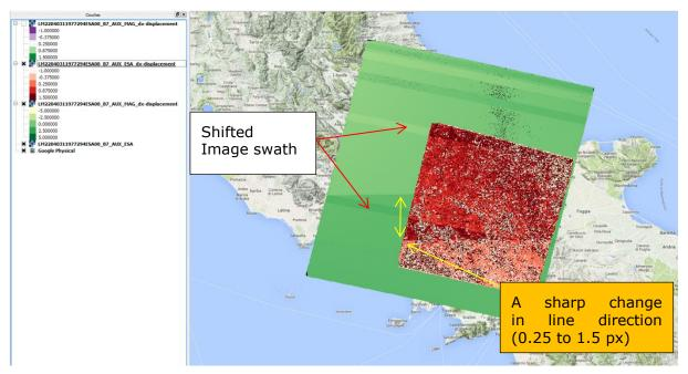
Figure 14- LS02 Image deformations (L8 and 'SV\_PRE'), LM22040311977294ESA00.
