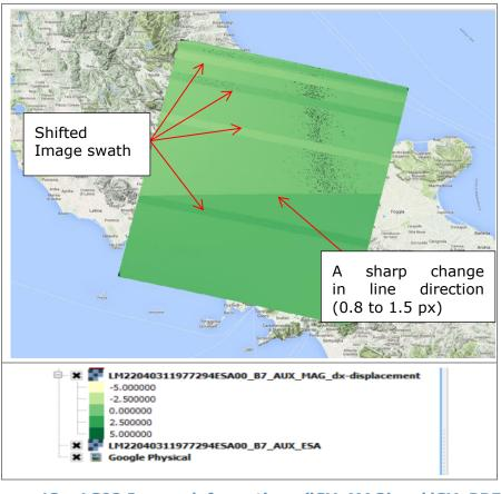
Figure 13 – LS02 Image deformations ('SV\_MAG' and 'SV\_PRE'), LM22040311977294ESA00.
