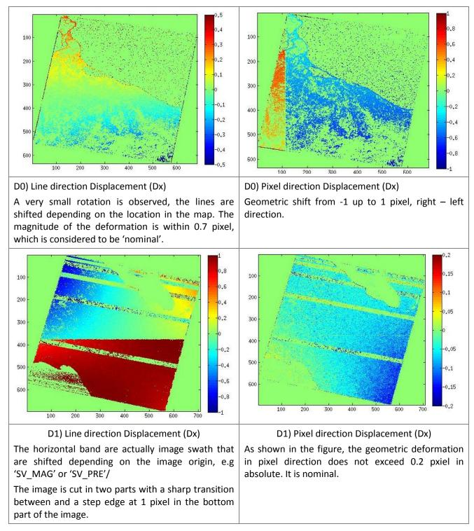
Figure 10 - LM22040371976336ESA00, GTC products, 'SV\_MAG' / 'SV\_PRE' image comparison.
