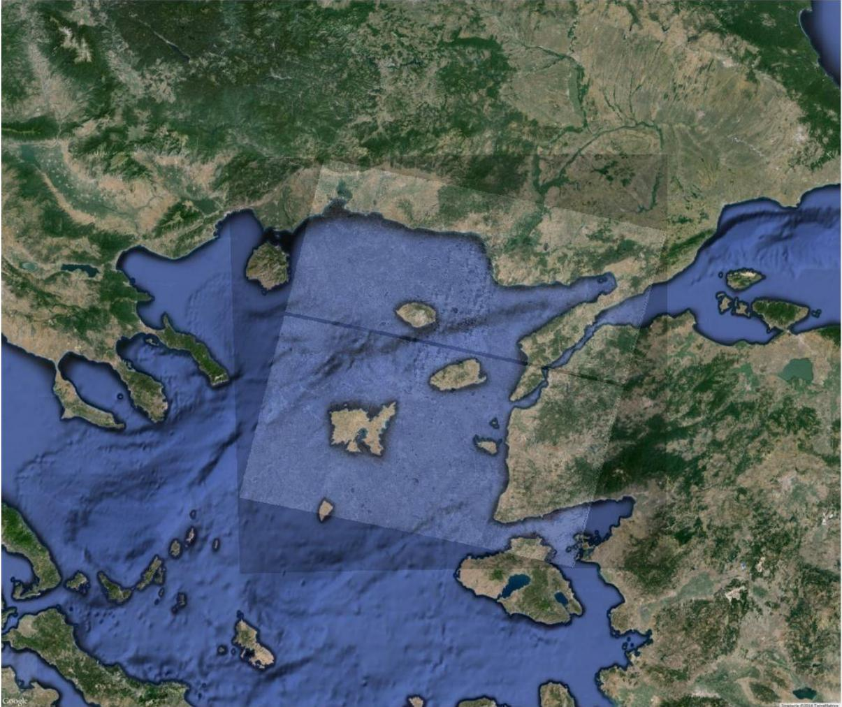
**fig 9.** *By applying image transparency, the mis registration is evident.*
